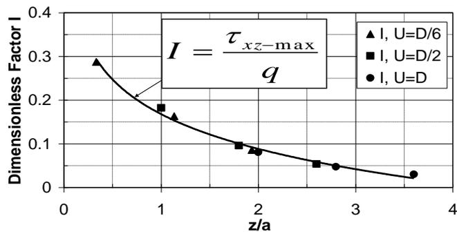
Figure (20) (Z/a)-I Relationship for the Location of Maximum Shear Stress [Mekkiyah (2003)] [6].
