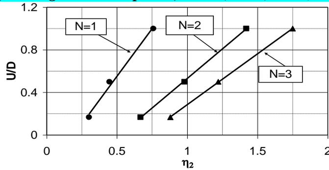
Figure (16) U/D versus Reduction Factor ( $\eta_2$ ) for Netlon CE121 [Mekkiyah (2003)] [6].
