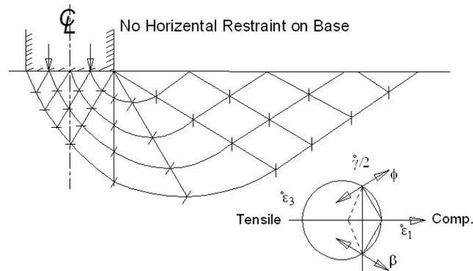
Figure (1) Zero extension characteristics for dilating soil (After Bassat and Last, 1978) [9].
