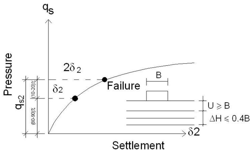
Figure( 4 ) Safe pressure ( $q_s$ ) for the settlement criterion of circular footing resting on reinforced subgrads ( $U \geq B$ ) [ Mekkiyah(2007) ] [7].
