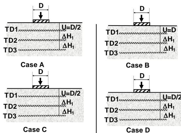
Figure (21) Developed Stress (TD) in the Reinforcement layers Under the Footing Based on the Method of Binquet and Lee [Mekkiyah (2003)] [6].
