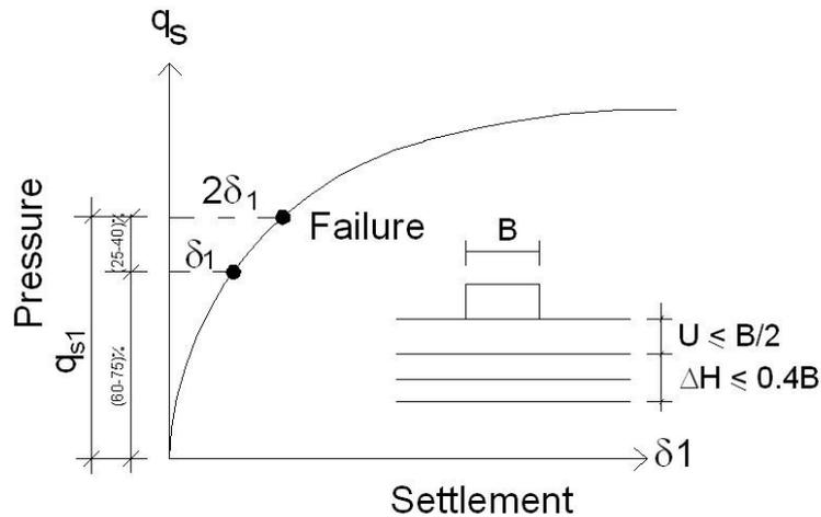
Figure (3) Safe bearing capacity ( $q_s$ ) for the settlement criterion of circular footing resting on reinforced subgrads ( $U \leq B/2$ ) [Mekkiyah (2007)] [7].
