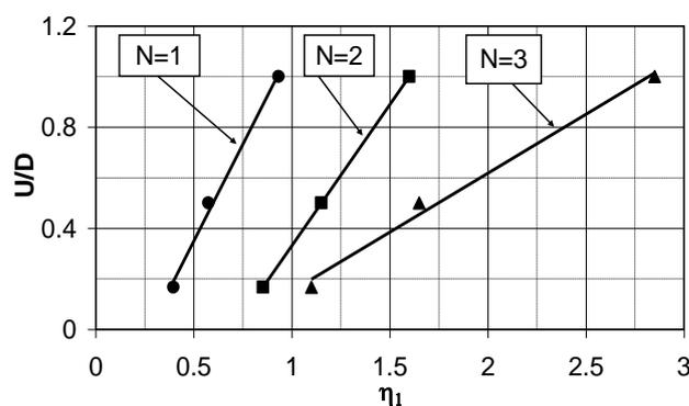
Figure (15) U/D Versus Reduction Factor ( $\eta_1$ ) for Netlon CE111[Mekkiyah(2003)] [6].
