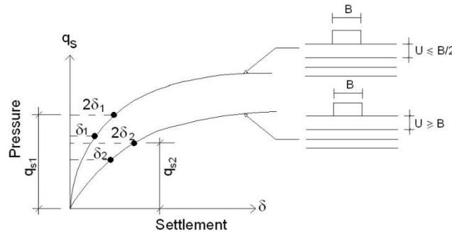
Figure (5) Safe bearing capacity ( $q_s$ ) for the settlement criterion for RFS ( $U \leq B/2$  and  $U \geq B$ ) reinforced subgrads) [Mekkiyah (2007)] [7].
