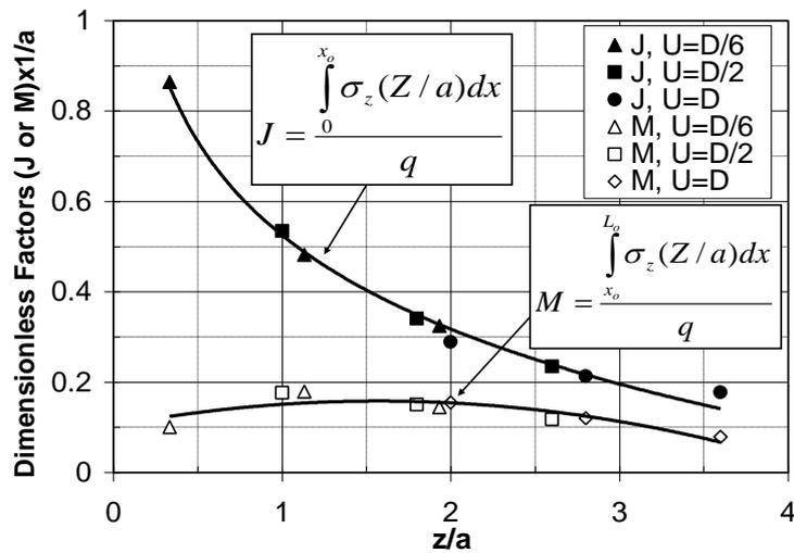
Figure (19) (Z/a)-J or M Relationship for the Effect of Vertical Stress [Mekkiyah (2003)] [6].
