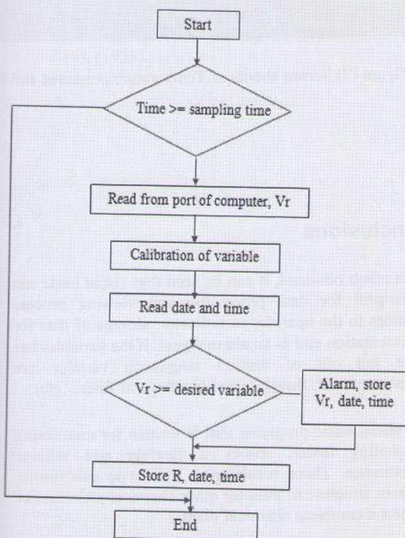
Figure (2) Algorithm of Program Reading
