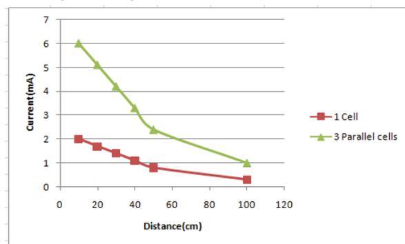
Figure 3. Current Characteristics of an Indoor Solar Cell
