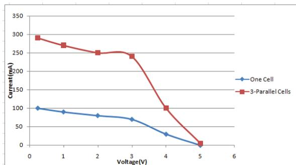
Figure 1. Measured V-I characteristics of the Solar World 4-4.0-100 solar panel
