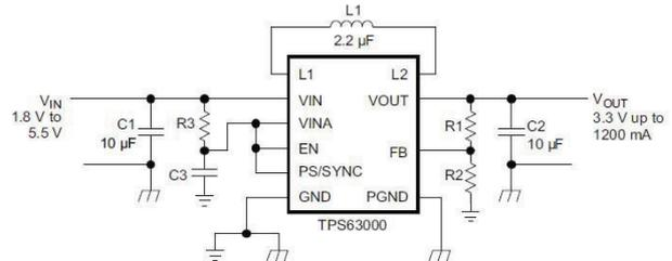
Figure 4. Application Circuit for Adjustable Output Voltage Option
