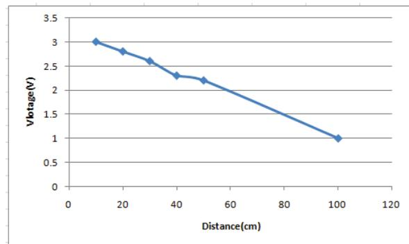
Figure 2. Voltage Characteristics of an Indoor Solar Cell
