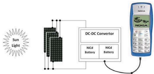
Figure 6. The Suggested Solar Energy Harvesting Circuit
