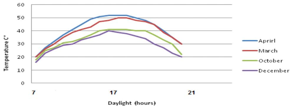
**Fig.(8) Temperature of the water during daylight hours For the different months of the year**
