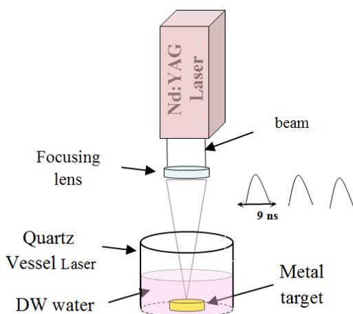
Fig. (1) Schematic diagram of laser ablation setup
