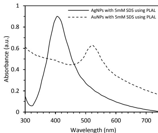
Fig. (2) Absorption spectra of (a) Ag nanoparticles and (b) Au nanoparticles synthesized by pulsed laser ablation technique in 5mM SDS
