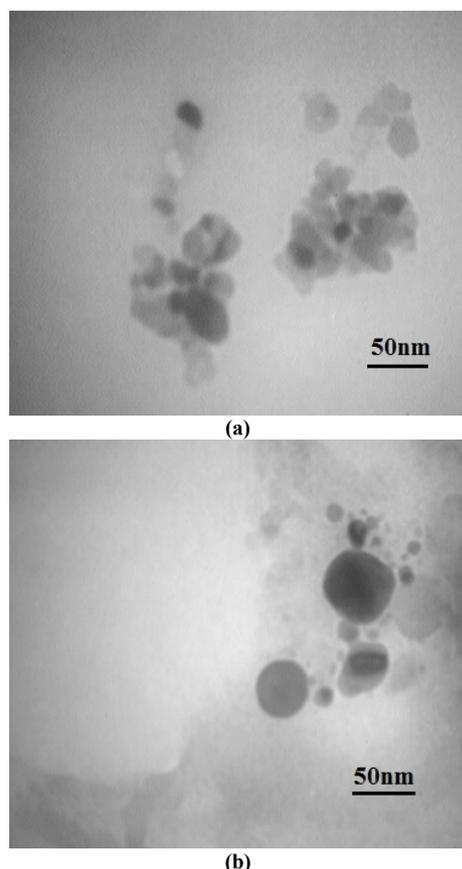
Fig. (4) TEM images of (a) gold (Au) nanoparticles and (b) silver (Ag) nanoparticles, obtained by PLAL of metal plates immersed in DW with SDS surfactant solution using 400 pulses of Nd:YAG laser
