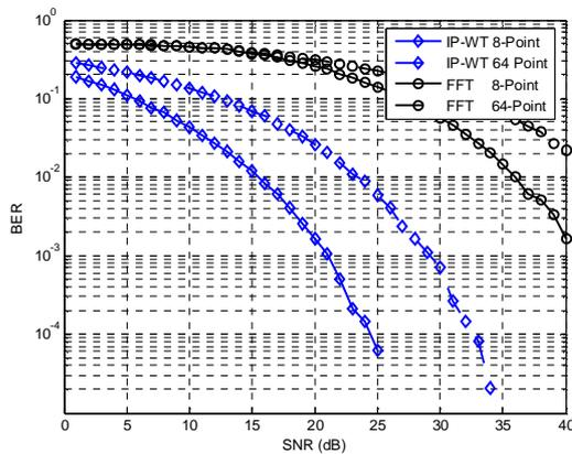
Fig. 7 Performance of the proposed and traditional OFDM in flat fading channel (maximum Doppler shift=5 Hz).
