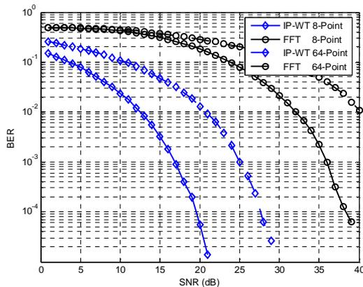
**Fig. 4 BER performance of the proposed OFDM based IP-WT and the traditional model based FFT in AWGN channel.**
