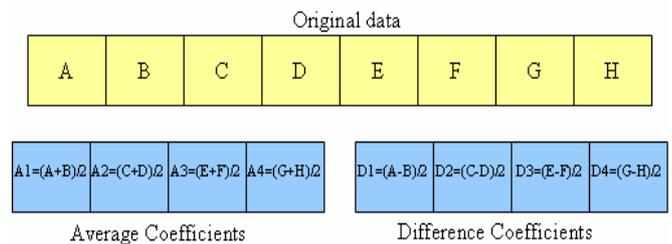
Fig. 1 Forward Haar transform for an 8-coefficient row.
