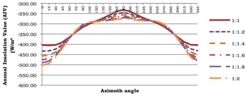
**Figure 7:** Annual Insolation Value (AIV) of iwan with different D:W ratios and in different orientations. (Source: Researchers)
