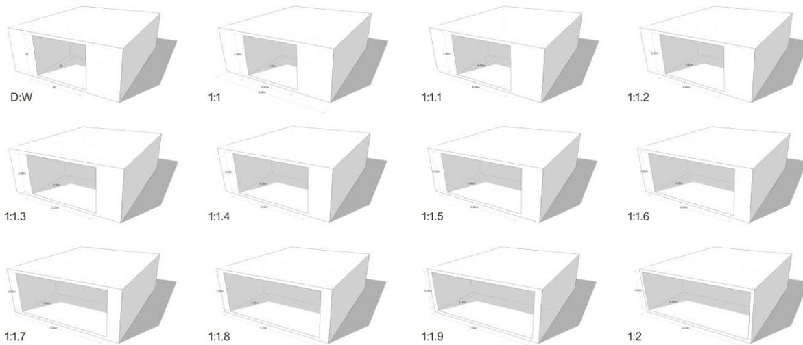
**Figure 2:** 3D models of considered iwan proportions in simulations.
