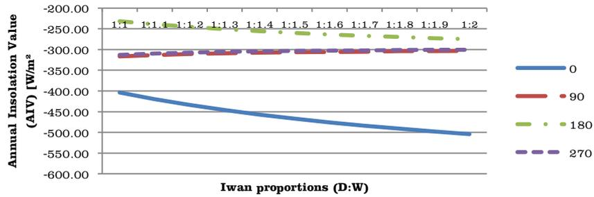
**Figure 6:** Annual Insolation Value (AIV) of iwan in different orientations and with different D:W ratio. (Source: Researchers)
