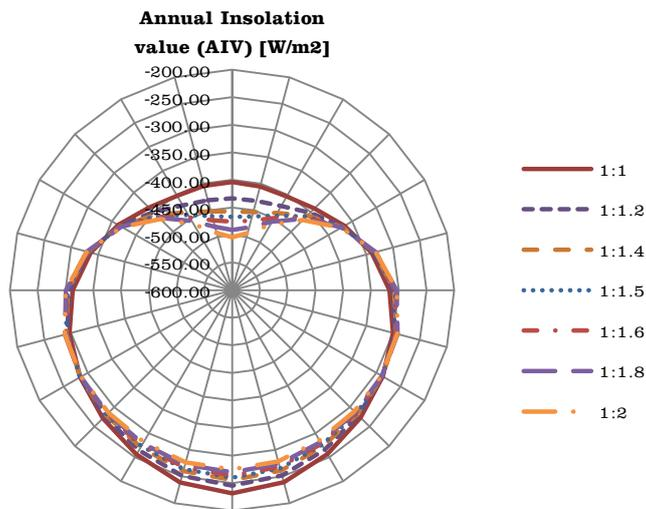
**Figure 8:** Annual Insolation Value (AIV) of iwan with different D:W ratios and in different orientations. (Source: Researchers)
