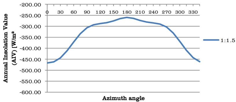
**Figure 4:** Annual Insolation Value (AIV) of an iwan with D:W ratio of 1:1.5 and in different orientations. (Source: Researchers)
