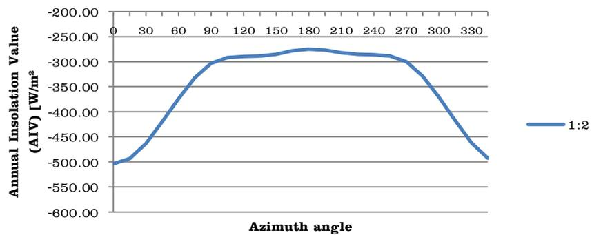
**Figure 5:** Annual Insolation Value (AIV) of an iwan with D:W ratio of 1:2 and in different orientations. (Source: Researchers)
