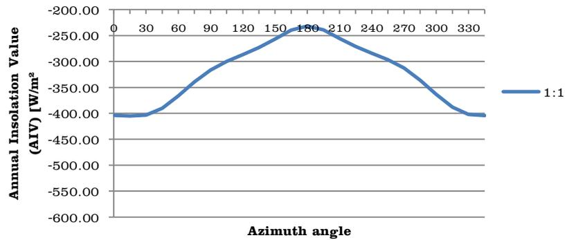
**Figure 3:** Annual Insolation Value (AIV) of an iwan with D:W ratio of 1:1 in different orientations. (Source: Researchers)
