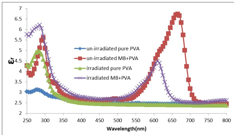
**Fig.(8)** The real part of dielectric constant for un-irradiated and irradiated pure PVA and MB/PVA films
