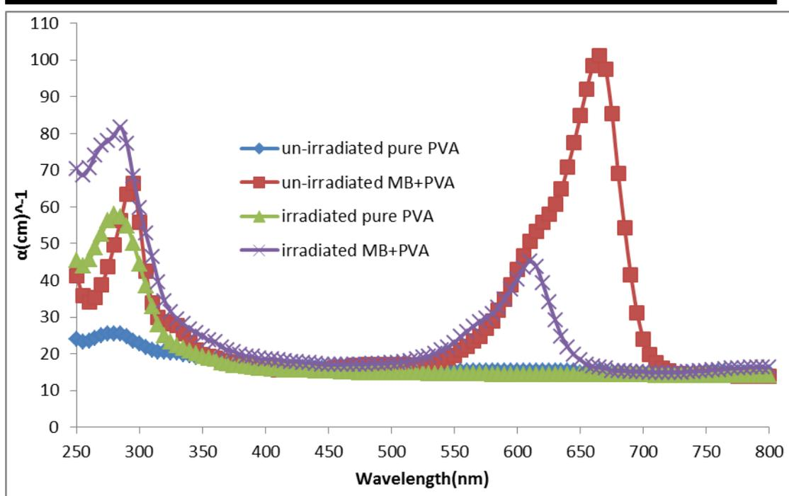
**Fig.(4)** the absorption coefficient for un-irradiated and irradiated pure PVA and MB/PVA films
