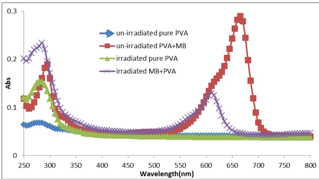
**Fig.(1)** The absorption spectrum of un-irradiated and irradiated pure PVA and MB/PVA films
