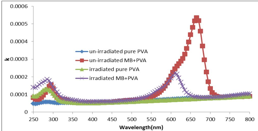
Fig.(6) The extinction coefficient for un-irradiated and irradiated pure PVA and MB/PVA films
