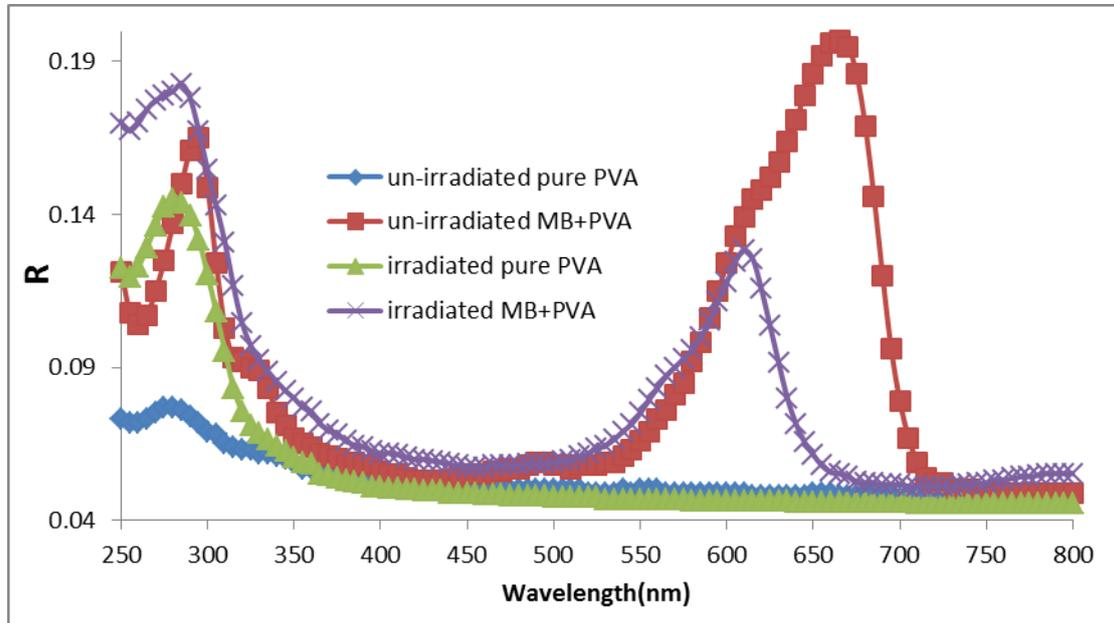
**Fig.(3)** The reflectance for un-irradiated and irradiated pure PVA and MB/PVA films
