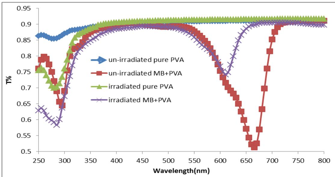
**Fig.(2)** The transmission spectrum for un-irradiated and irradiated pure PVA and MB/PVA films
