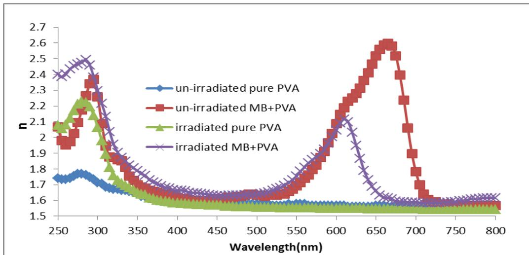
Fig.(7) The refractive index for un-irradiated and irradiated pure PVA and MB/PVA films
