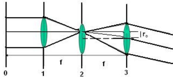
Figure( 6) Keplerian Afocal telescopic type scanner system
