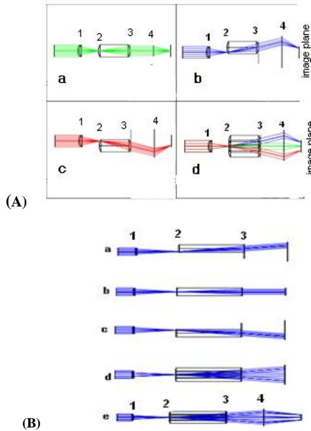
Figure (7) Designed Keplerian telescopic Afocal micro scanner system for maximum scan angle, (A)  $F_{\#} 1.5$ , (B)  $F_{\#} 5$  [1focusing lens, 2 Mid lens and 3 last lens on the same substrate, 4 is an imaging lens] , where for both A & B a)  $r_o = +0.04\text{mm.}$ , b)  $r_o = 0.0\text{mm.}$ , c)  $r_o = -0.04\text{mm.}$ , d) at all scanning angles  $r_o = 0, \pm 0.04\text{mm.}$ , e) for B with imaging lens 4.
