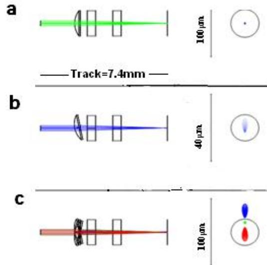
Figure (3) Layout of single aperture micro scanner(case 1, ENPD=0.3mm,  $\lambda = 1.064\mu\text{m}$ ), a) at  $0^\circ$  tilt angle, b) at  $+11.5^\circ$  tilt angle, c) at all tilt angles, on the right are shown spot diagrams at the image plane surrounded by the Airy disc .
