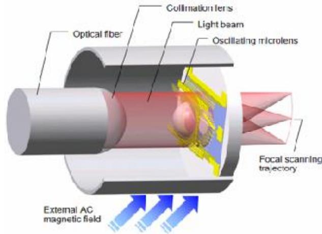
Figure (2) Schematic of single aperture micro scanner system[7].
