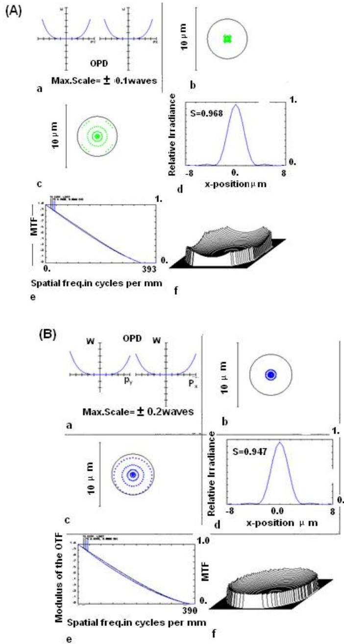
Figure (8) Characteristics curves of micro keplerian telescopic system with  $F\#5$ , for (A)  $r_o=0.0\text{mm}$  (B)  $r_o=0.04\text{mm}$ , where in both A & B a) OPD at image plane, b) spot diagram at mid focusing plane, c) spot diagram at image plane, PSF with Strehl ratio  $S = 0.968$  in A &  $S=0.947$  in B, e) MTF curve, f) wavefront map.
