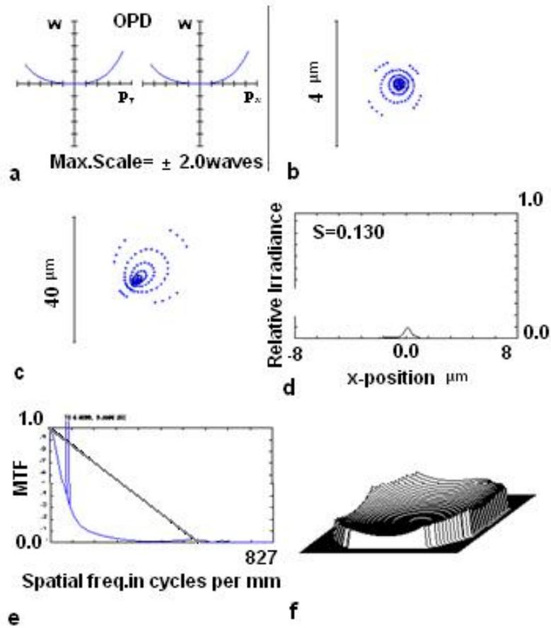
Figure (9) Characteristics curves of Keplerian micro telescopic system with  $F_{\#}$  1.5, for  $r_o=0.04\text{mm}$ , a) OPD at image plane, b) spot diagram at mid focusing plane, c) spot diagram at image plane, d) PSF with Strehl ratio=0.130, e) MTF curve, f) wavefront map.
