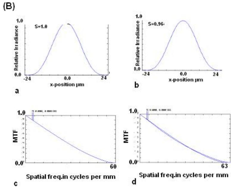
Figure (4) Characteristics curves of single aperture scanner (case 1, ENPD=0.3mm,  $\lambda=1.06 \mu\text{m}$ ) (A) - a)OPD at  $0^\circ$  tilt angle, b) OPD at  $+11.5^\circ$  tilt, c) wavefront map at  $0^\circ$  tilt, d) wavefront map at  $+11.5^\circ$  tilt . (B) - a)PSF at  $0^\circ$  tilt, b)PSF at  $+11.5^\circ$  tilt, c) MTF at  $0^\circ$ ,d) MTF at  $+11.5^\circ$ .
