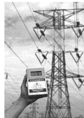
Fig.(4) :Electromagnetic field tester (EMF tester) type band pass ac gauss meter
