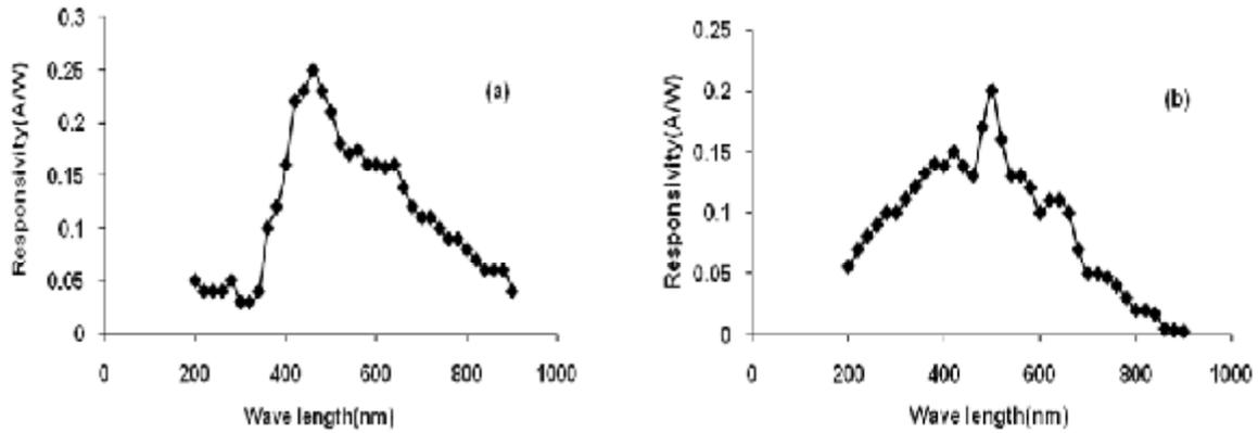
Figure (6): Spectral responsivity as a function of incident photon wavelength (a) (Al/MgO/Si) (b) (Al/SiO<sub>2</sub>/Si) devices.
