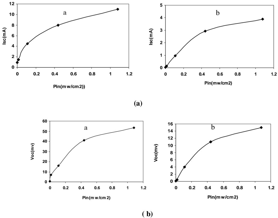
Figure 5(a) Short circuit current and (b) open circuit voltage as a function of the incident photo energy for (Al/MgO/Si), (Al/SiO<sub>2</sub>/Si) MOS devices respectively.
