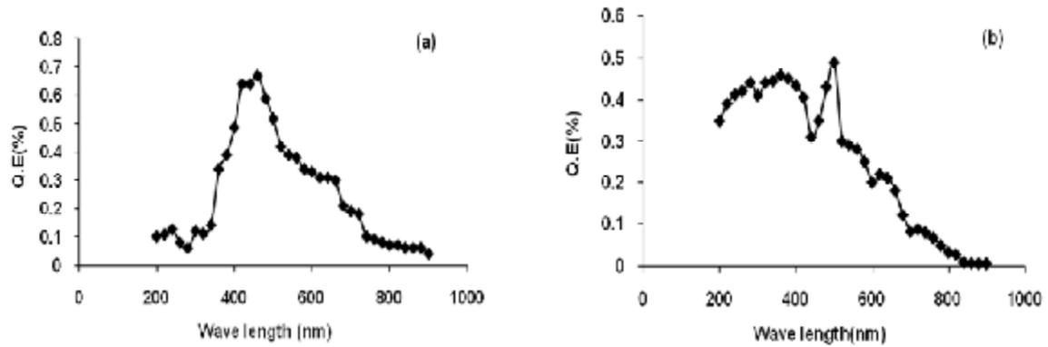
Figure (7): Quantum efficiency as a function of incident photo wavelength (a) (Al/MgO/Si), (b) (Al/SiO<sub>2</sub>/Si)
