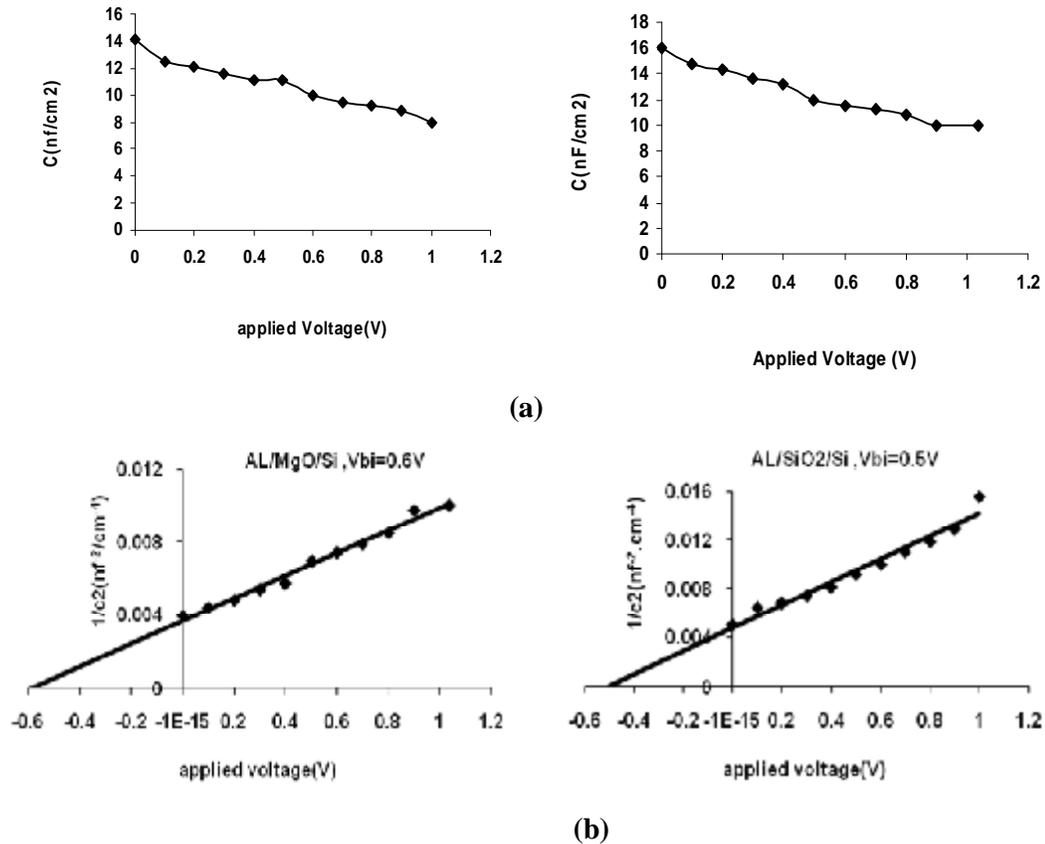
Figure 3 (a) Junction capacitance as a function of the applied voltage for ( b)  $1/C^2$  vs. applied voltage for (Al/MgO/Si), (Al/SiO<sub>2</sub>/Si) MOS device respectively.
