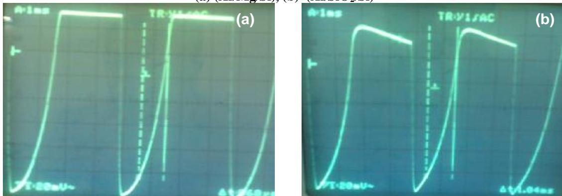
Figure (8): The response time as a function of the rise time (a) (Al/MgO/Si), (b) (Al/SiO<sub>2</sub>/Si)
