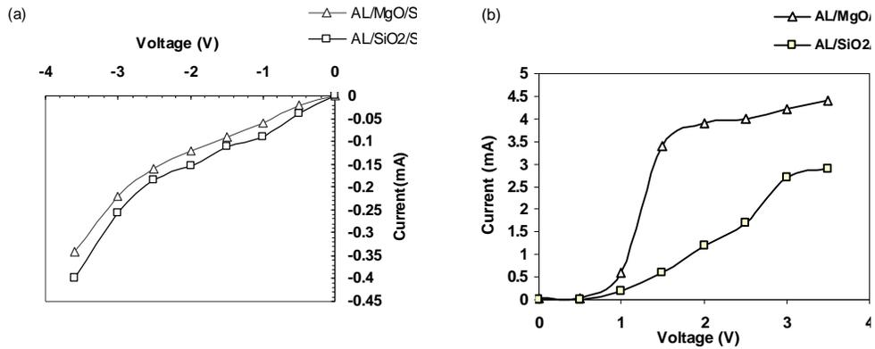
Figure 2(a,b) I-V characteristic under forward and reverse bias of the both MOS Devices.
