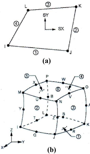
Fig.3, Element Geometry; (a) Plane 42, (b) SOLID 95.
