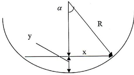
**Fig.1, Geometry of Cam-Follower Contact Near Circular Limit.**
