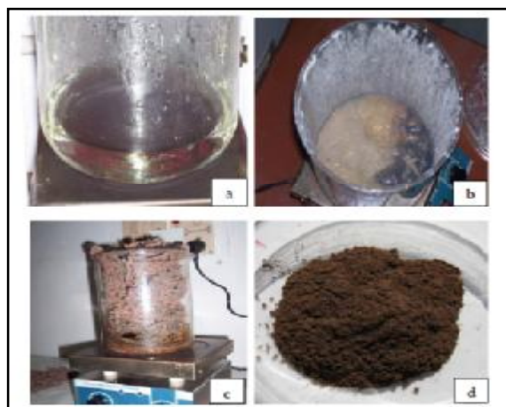
Figure (1) Photograph of (a) nitrate-citrate solution, (b) dry gel, (c) Auto combustion reaction and (d) burnt ash powder.
