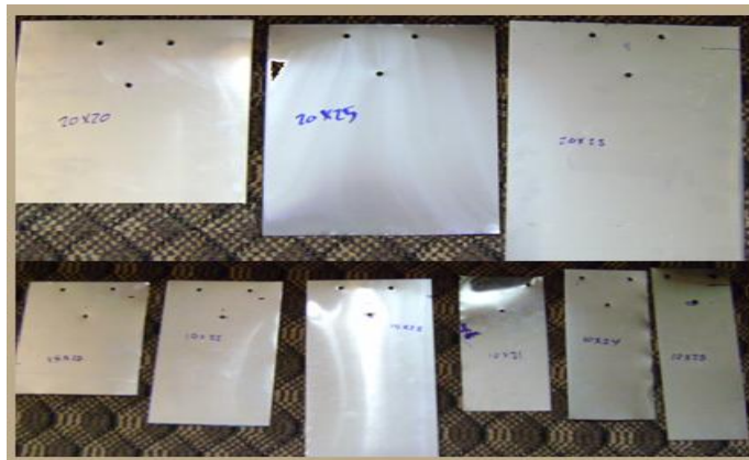
Figure (3) Nine test samples of cantilever plates
