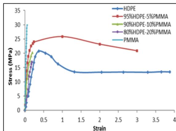
Figure 3: Stress-strain curve of HDPE-PMMA polymer blends
