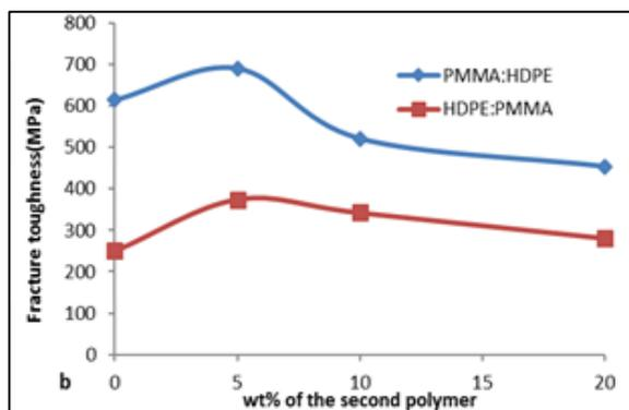
Figure 6: Fracture toughness of polymer blends (PMMA: HDPE) and (HDPE: PMMA)
