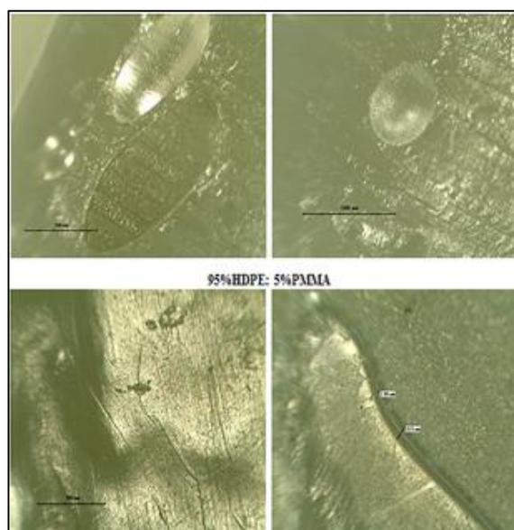
Figure 8: Optical micrographs of (HDPE: PMMA) polymer blends
