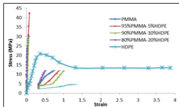
Figure 2: Stress-strain curve of polymer blends (PMMA: HDPE)
