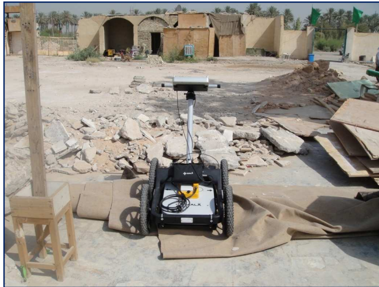
Figure (1) MALA GPR System used in the site location of study area
