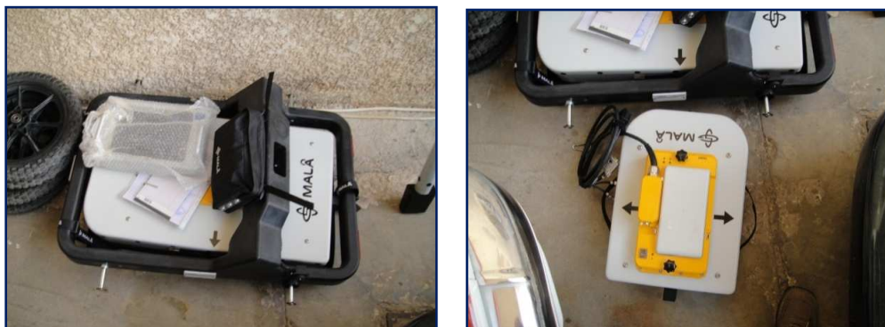
Figure (2) MALA GPR Instrument part (Antenna, Control Unit, Monitor)
