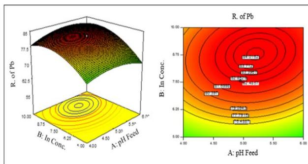
Fig. 4. Interacting effects of pH feed and Carrier concentration on lead removal: surface plot; contour plot
