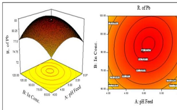
Fig. 3. Interacting effects of pH feed and initial metals concentration on lead removal: surface plot; contour plot
