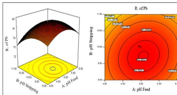
Fig. 2. Response surface plot, Contour plot of the Interacting effects of pH feed and pH stripping on lead removal
