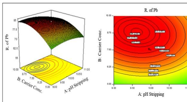
Fig. 6. Interacting effects of pH stripping and Carrier concentration on lead removal: surface plot; contour plot
