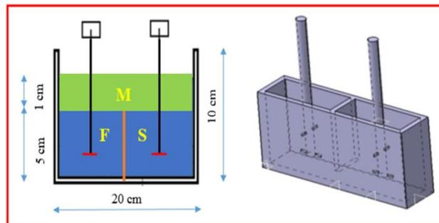
Fig. 1. Bulk liquid membrane system used in this work
