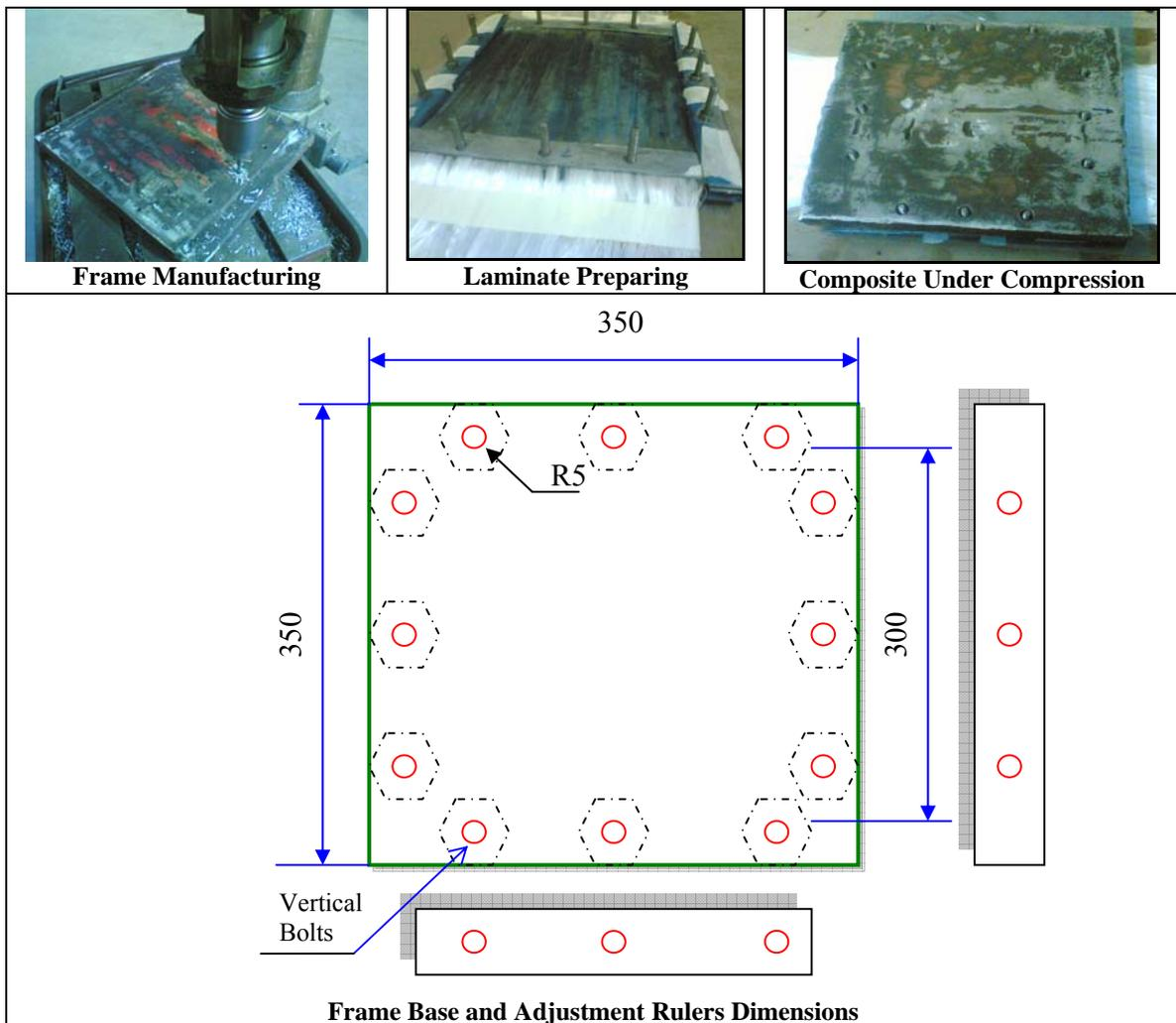
Figure (1) Manufacturing Process and Frame Dimensions
