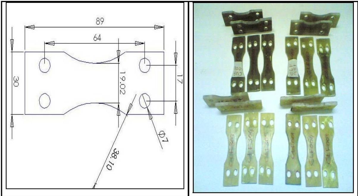
Figure (2) Fatigue Specimens (all dimension in mm)
