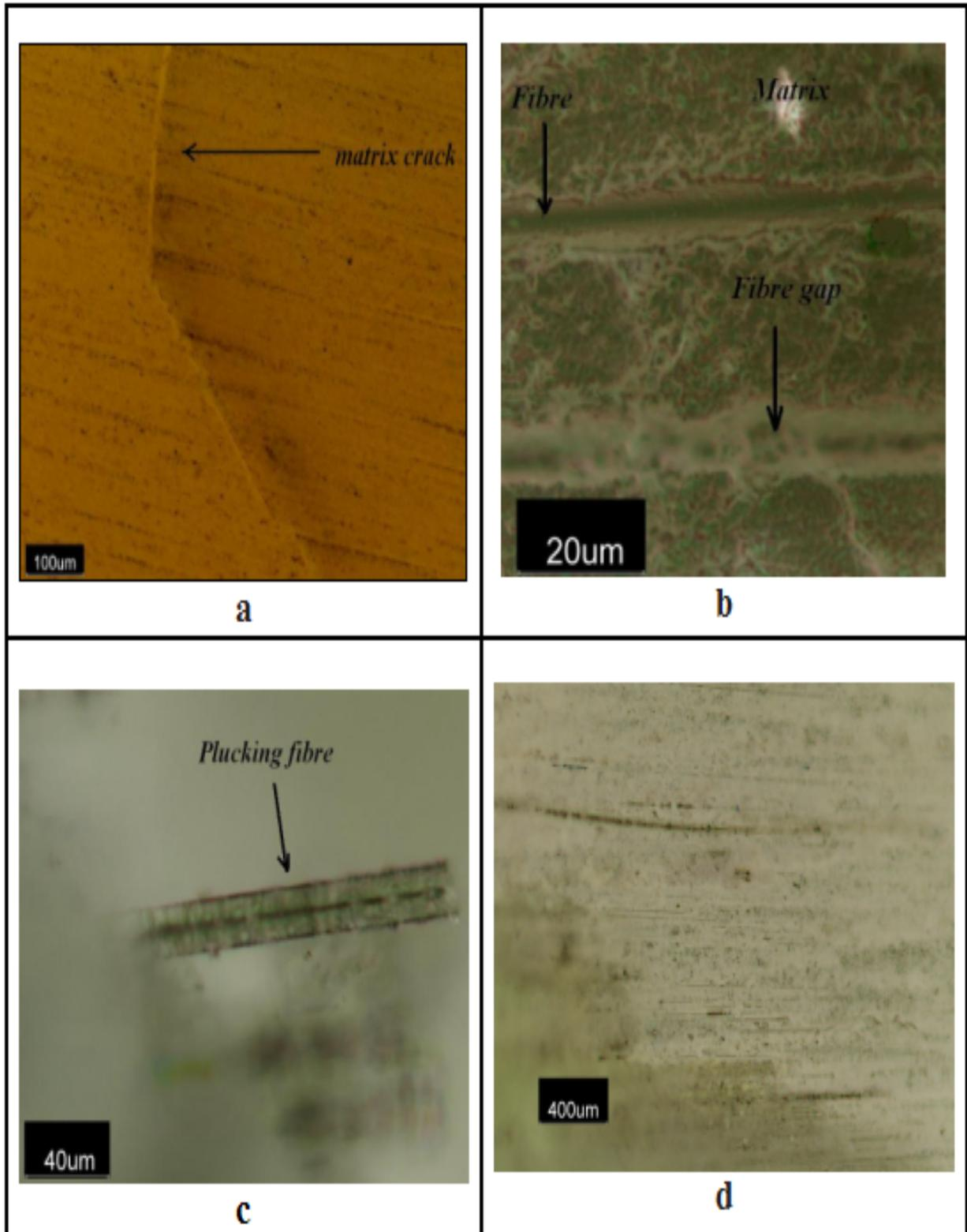
Figure (4) Micrographs of Fatigue Failure Observed in Glass Polyester Composites.
