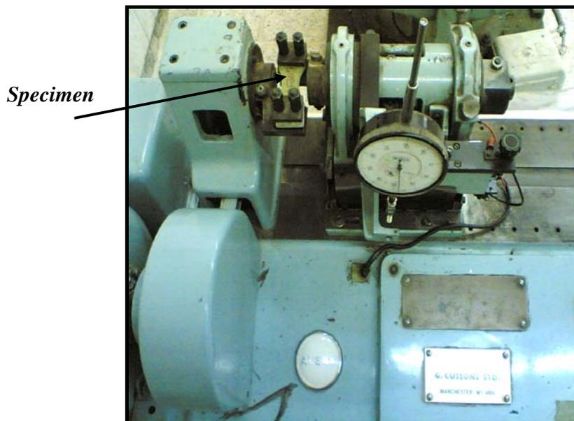
Figure (3) AVERY Fatigue Testing Machine Type 7305
