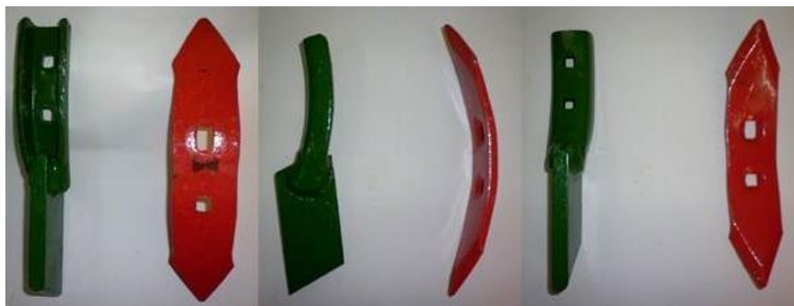
Fig (3) Different between ZT seeder tine (green) and normal seeder bird tongue tine
