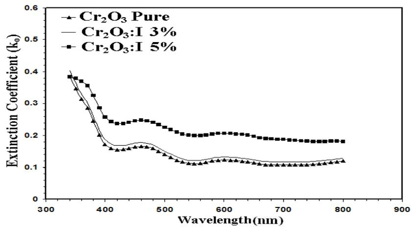
Fig (4): Extinction coefficient against wavelength for the undoped and I-doped ( $\text{Cr}_2\text{O}_3$ ) thin films.
