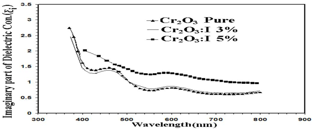
Fig (7): Imaginary part of dielectric constant against wavelength for the undoped and I-doped (Cr<sub>2</sub>O<sub>3</sub>) thin films.
