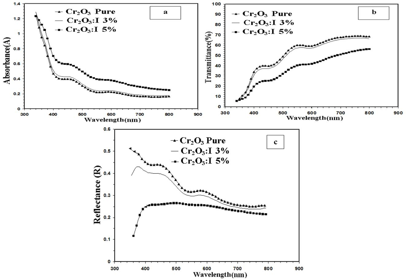
**Fig(1):(a) Absorbance (b)Transmittance (c)Reflectance spectra against wavelength of the undoped and I-doped ( $\text{Cr}_2\text{O}_3$ ) thin films .**
