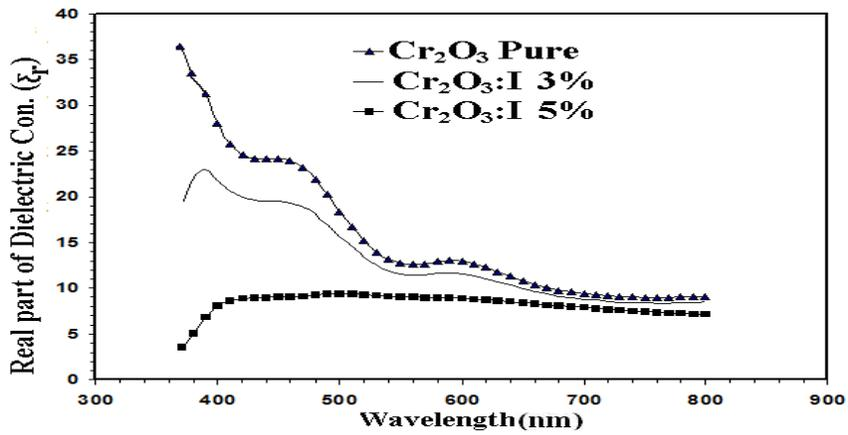
Fig (6): Real part of dielectric constant against wavelength for the undoped and I-doped (Cr<sub>2</sub>O<sub>3</sub>) thin films.
