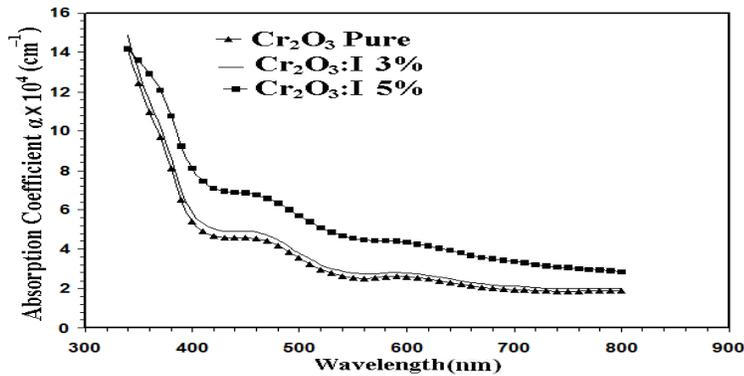
**Fig (2): Absorption Coefficient (a) against wavelength for the undoped and I-doped ( $\text{Cr}_2\text{O}_3$ ) thin films.**
