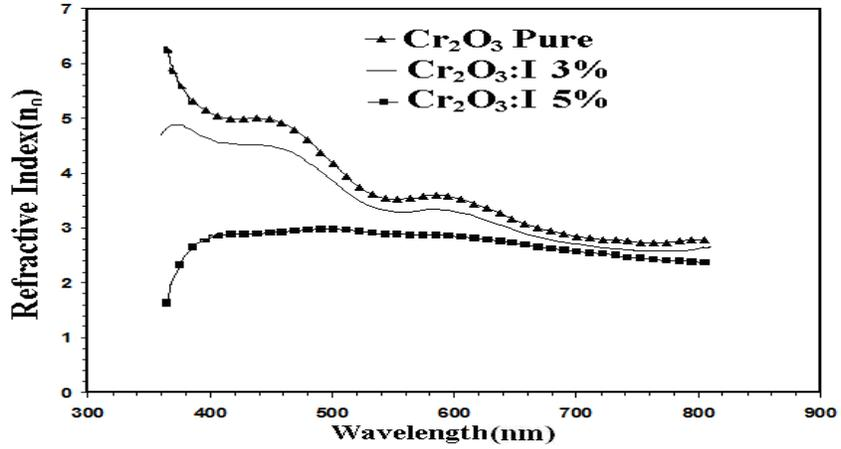
Fig (5): Refractive index against wavelength for the undoped and I-doped (Cr<sub>2</sub>O<sub>3</sub>) thin films.
