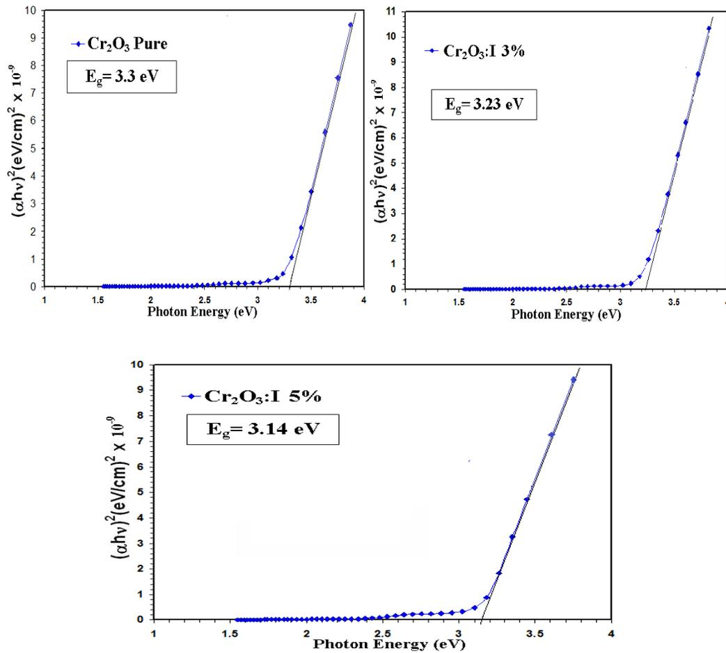
Fig (3):  $(\alpha h\nu)^2$  for the undoped and I-doped ( $\text{Cr}_2\text{O}_3$ ) thin films versus photon energy.
