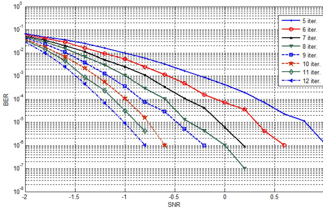
**Fig .(5) The performance of LDPC with various number of iteration**
