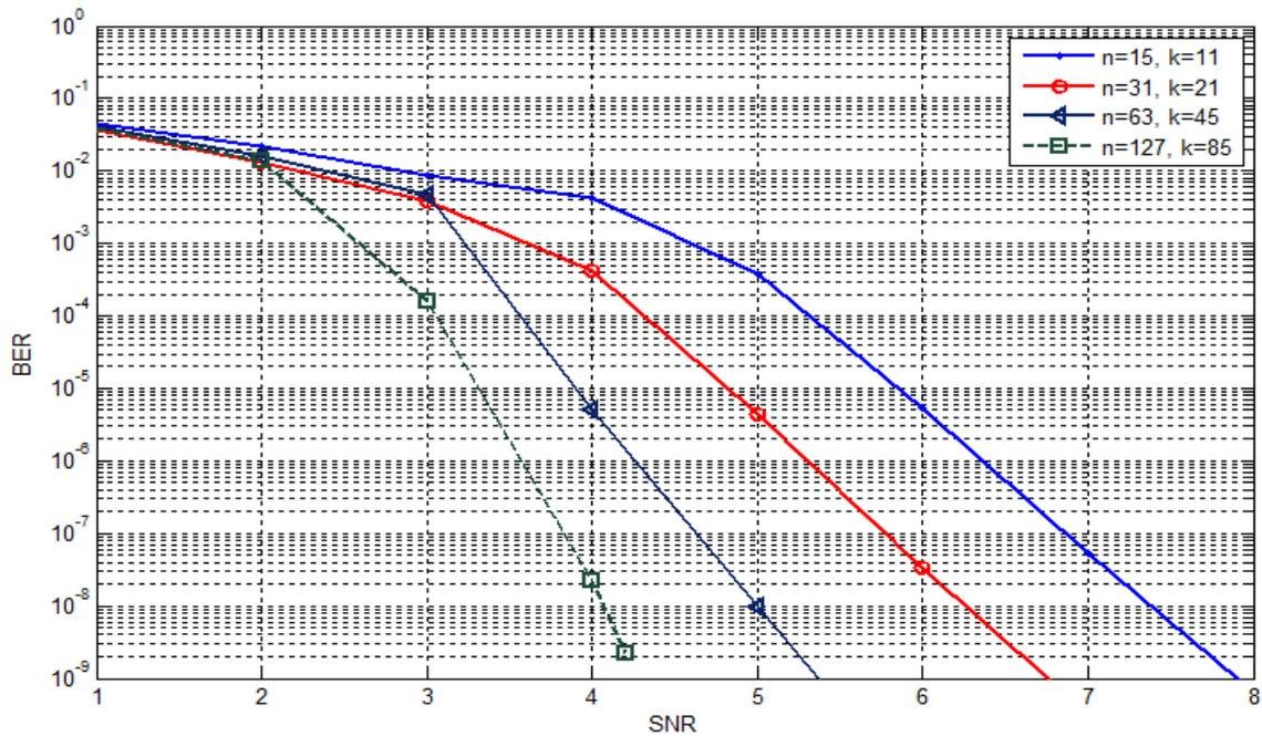
**Fig .(4) the performance of BCH code with various codeword and fixed code rate**
