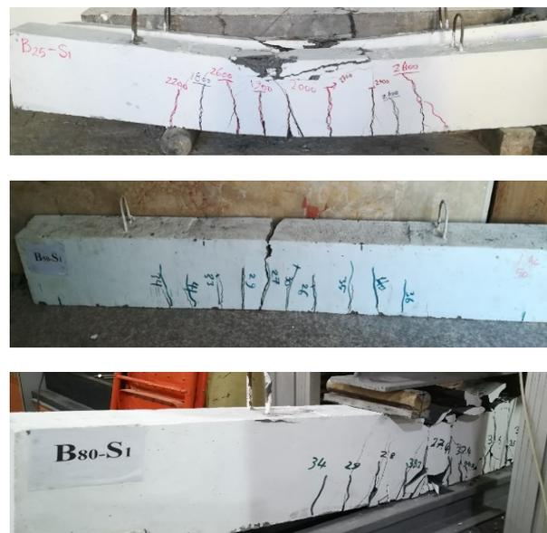
Figure 7: Cracks pattern of beams (25-S1.0), (50-S1.0), and (80-S1.0)
