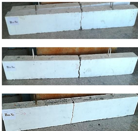
Figure 5: Failure of plain concrete beams
