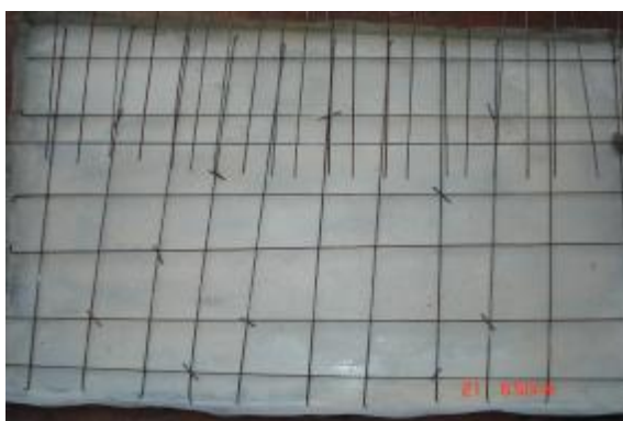
Photo (5) Details of the reinforcement mesh of slab S_6 (case6).
