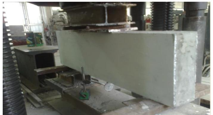
Figure (6) Photograph of a control rectangular deep beam with testing machine
