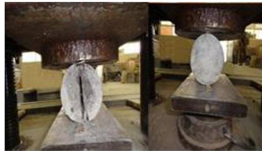
**Figure (3):Splitting tensile strength test**
