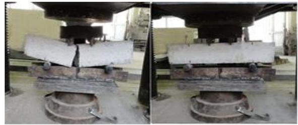
**Figure(2): Flexural strength test.**
