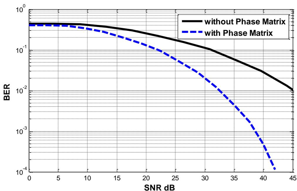
Fig.8. BER performance of proposed model in selective fading channel at maximum Doppler shift 500 HZ
