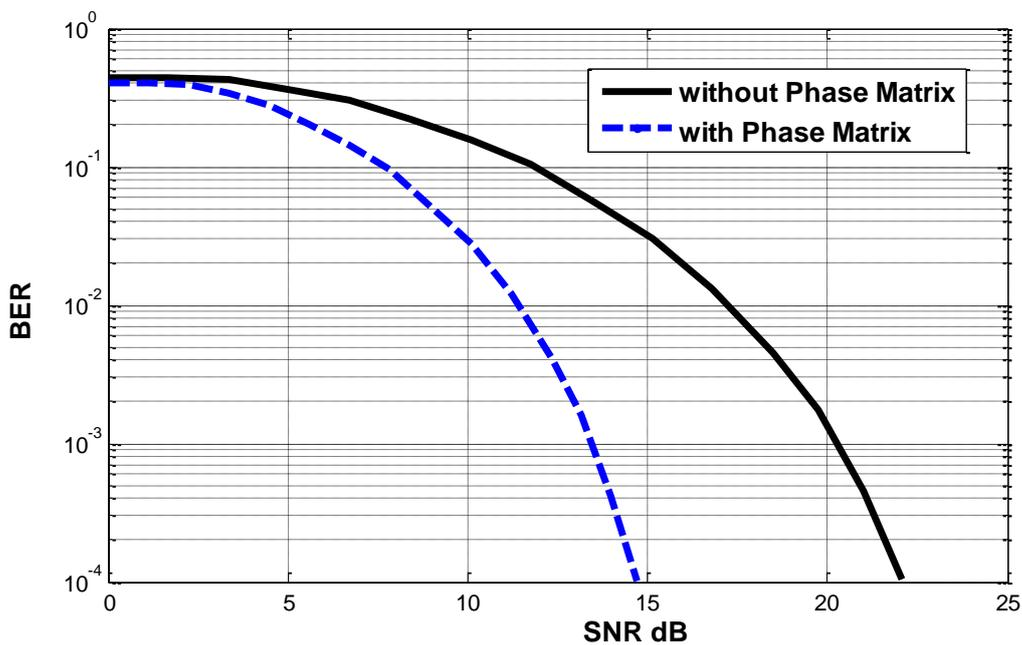
Fig.3. BER performance of proposed model in flat fading channel at maximum Doppler shift 10 HZ
