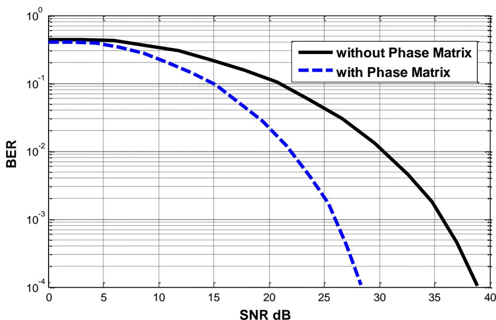
Fig.5. BER performance of proposed model in flat fading channel at maximum Doppler shift 500 Hz
