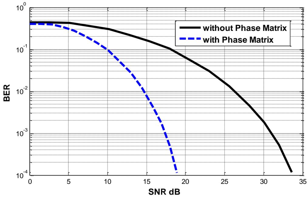
Fig.6. BER performance of proposed model in selective fading channel at maximum Doppler shift 10HZ
