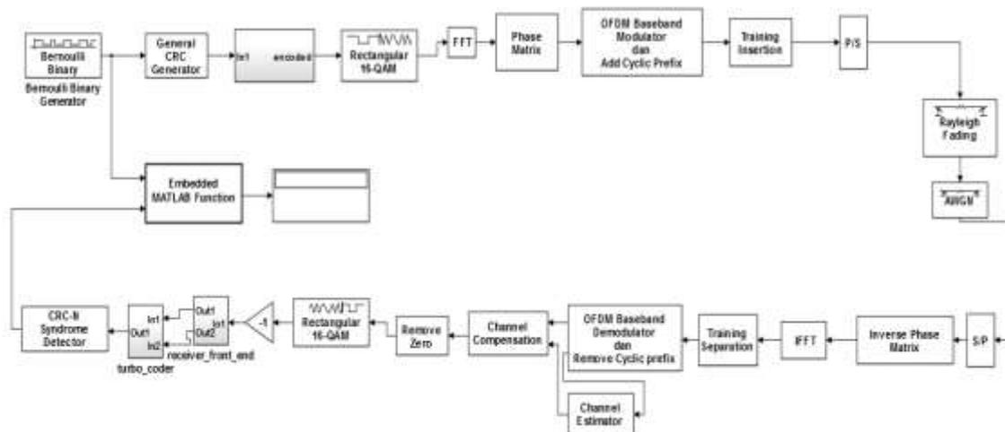
Fig. 1. Block Diagram of the Proposed LTE 3GPP Baseband Transceiver with Phase Matrix
