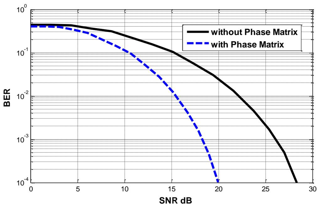
Fig.4. BER performance of proposed model in flat fading channel at maximum Doppler shift 100 HZ
