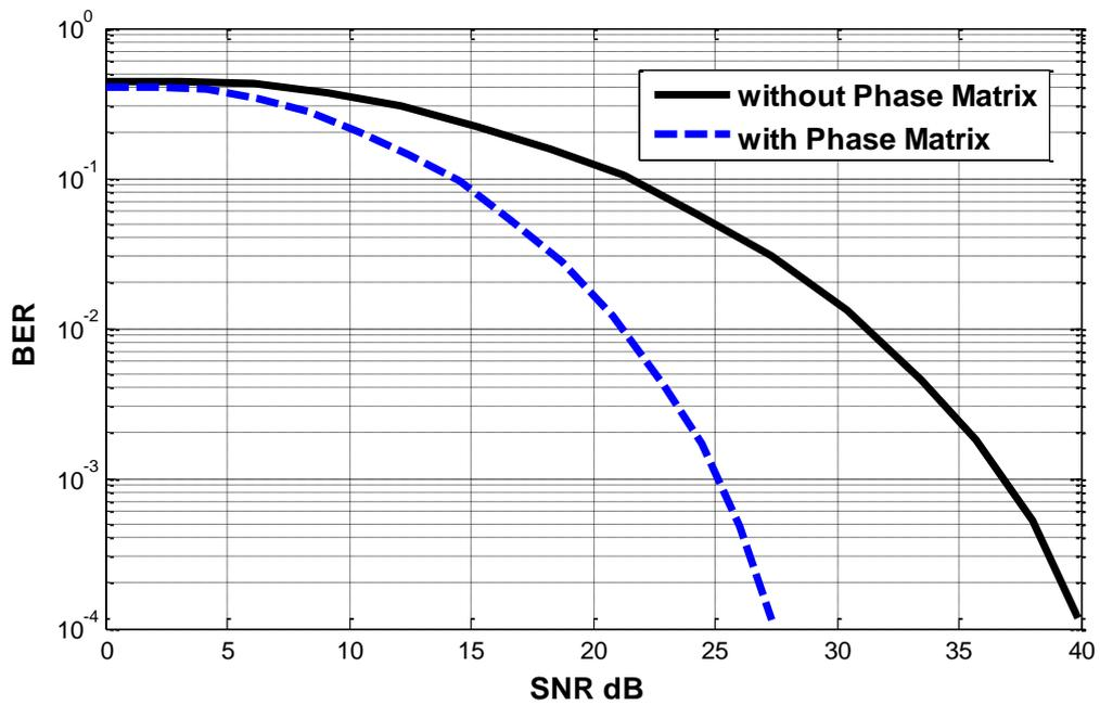
Fig.7. BER performance of proposed model in selective fading channel at maximum Doppler shift 100 HZ
