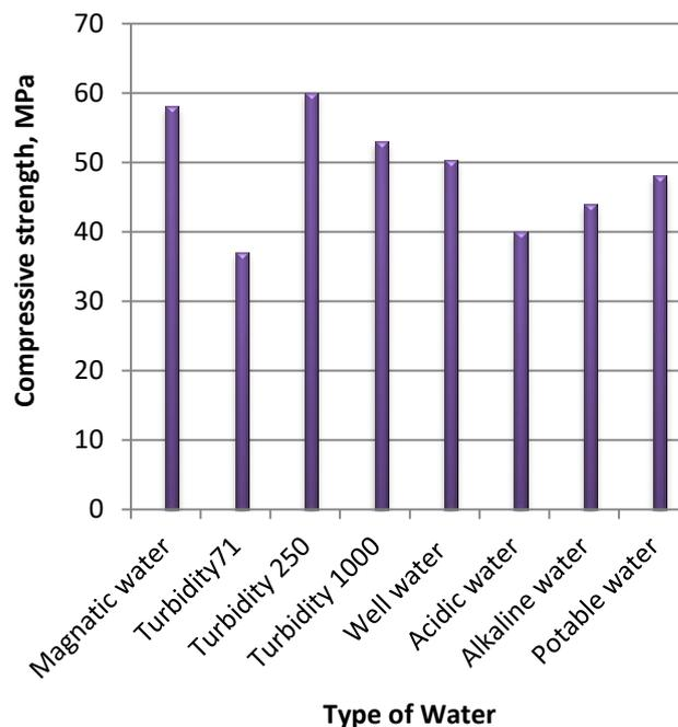
Figure 5: Variation of compressive strength with type of water at 28 days age
