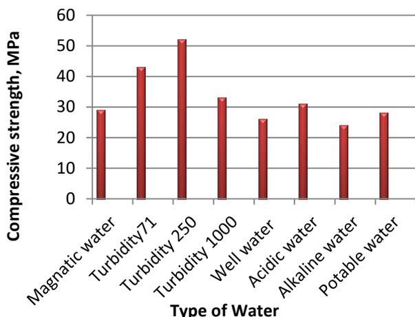
Figure 3: Variation of compressive strength with type of water at 7 days age
