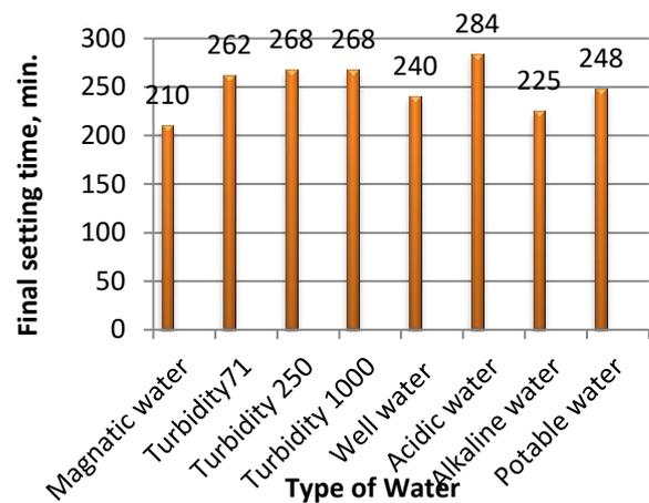
Fig. 2: Variation of final setting time with type of water
