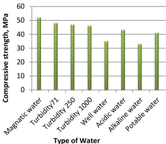
Figure 4: Variation of compressive strength with type of water at 14 days age
