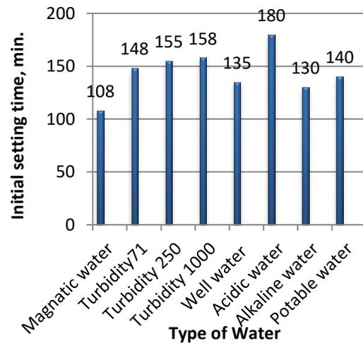
Fig. 1: Variation of initial setting time with type of water
