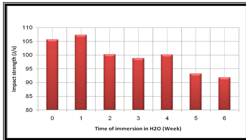
Fig.-1: Effect of H<sub>2</sub>O with Impact strength
