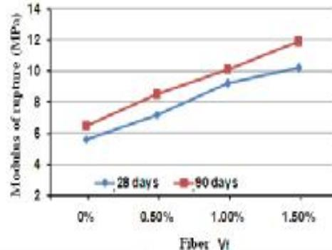
Figure (6): Effect of steel fiber content on the flexural tensile strengths of SCC.
