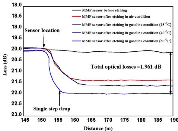
Fig. 10. The typical OTDR trace of MMF sensor response with unclad length 1 cm to temperature variation of gasoline condition.
