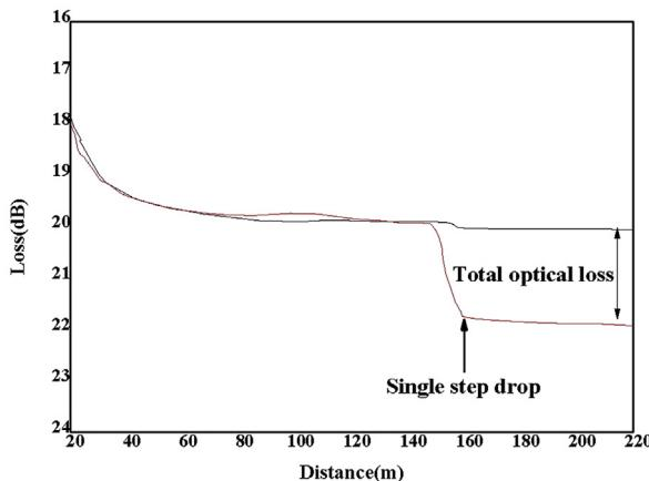
Fig. 6. OTDR trace attenuation showing the splicing loss, connector loss and Fresnel reflection.
