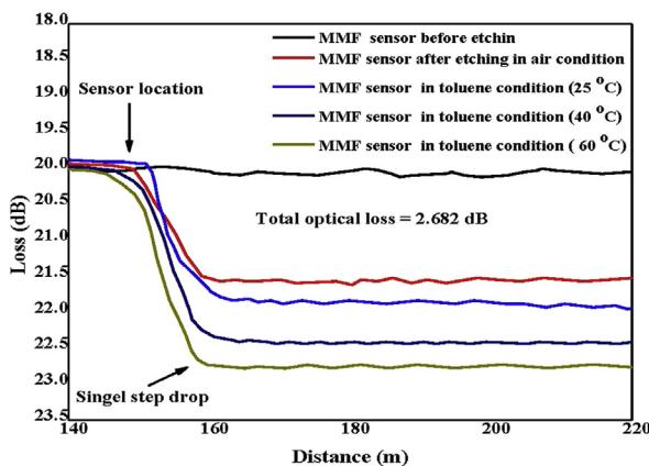
Fig. 11. The typical OTDR trace of MMF sensor response with unclad length 1 cm to temperature variation of toluene condition.
