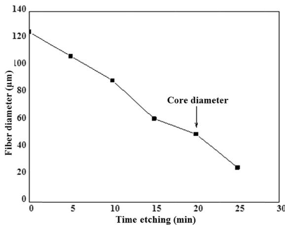
Fig. 4. The MMF sensor diameter against the etching time.
