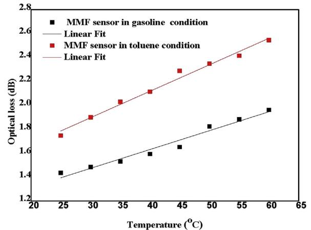
Fig. 12. Total optical loss versus the temperature variation of gasoline and toluene for 1 cm sensor.
