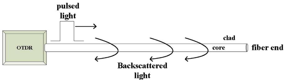
Fig. 1. Optical time domain reflectometry principle.
