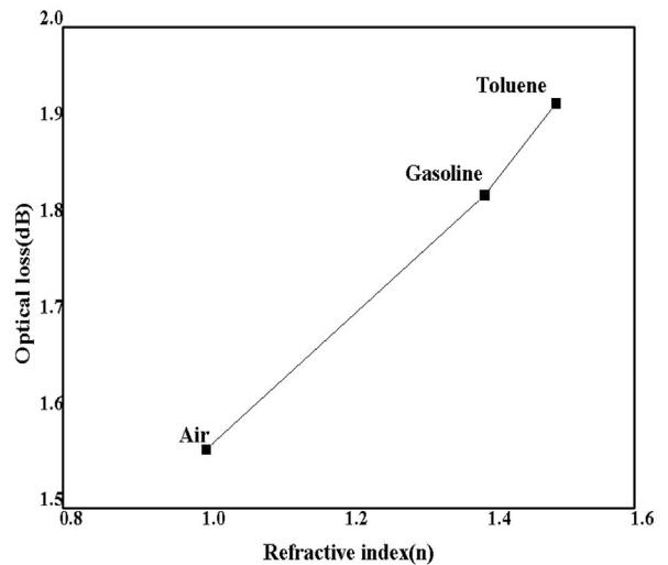
Fig. 8. The total optical loss versus refractive index (air, gasoline and toluene).
