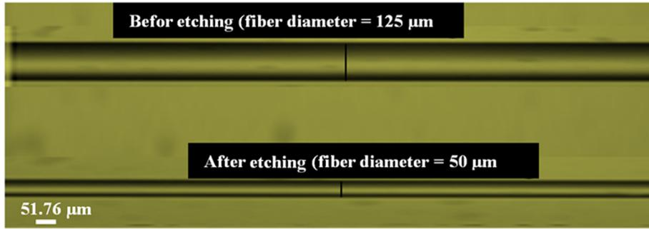
Fig. 3. Electron microscopic image of MMF sensor (before and after 20 min etching).
