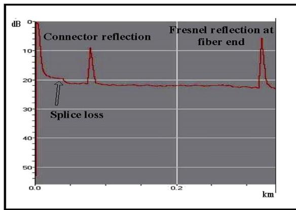
Fig. 2. OTDR trace attenuation includes the splicing loss, connector loss and Fresnel reflection.
