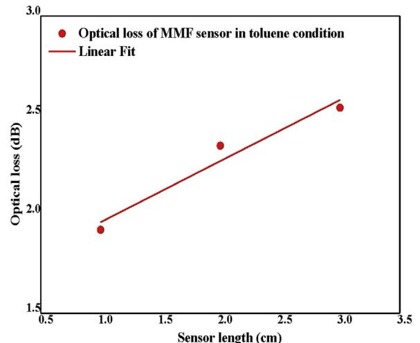
Fig. 9. The return loss versus different length of the MMF sensor immersed in toluene.
