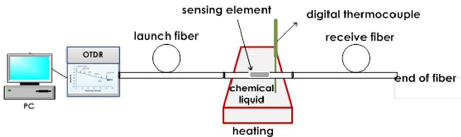
Fig. 5. The setup for temperature measurement using the MMF sensor.
