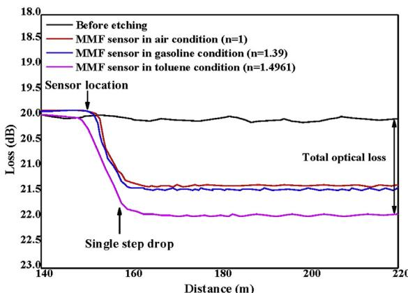
Fig. 7. The typical OTDR trace before etching and after 20 min etching 1 cm of unclad length of MMF sensor. The unclad part was exposed successively to gasoline and toluene.
