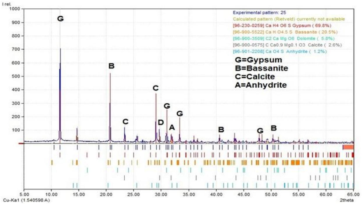
Fig. 2: X-Ray diffraction for gypsum rock in Zurbatiyah area.
