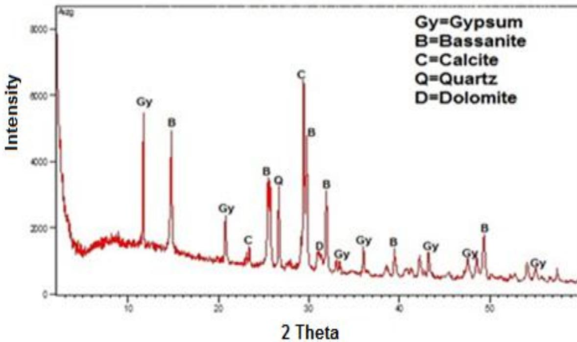
Fig.3: X-Ray diffraction for Zurbatiyah gypsum plaster
