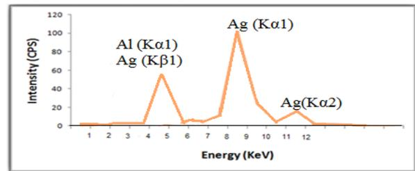
**Fig.(7) X-ray fluorescence of silver- alumina sample (face-1).**
