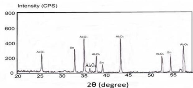
**Fig.(8) X-ray diffraction of Sn sample face2.**
