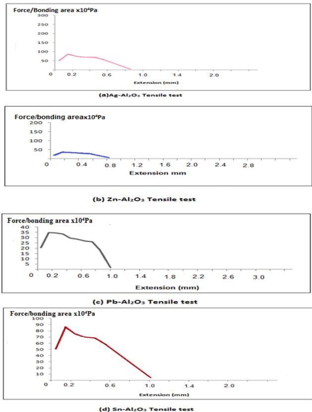
**Fig.(3) Typical Tensile tests for (a) Ag- $\text{Al}_2\text{O}_3$ . (b) Zn- $\text{Al}_2\text{O}_3$ . (c) Pb- $\text{Al}_2\text{O}_3$ .(d) Sn- $\text{Al}_2\text{O}_3$ .**
