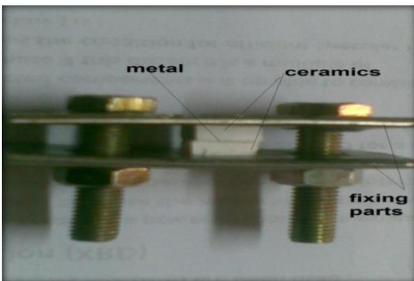
**Fig.(1) Joining Fixture Set up.**
