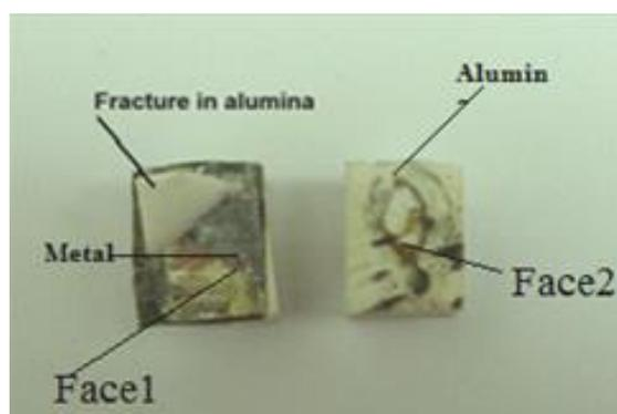
**Fig.(5) The fracture in alumina part for Ag sample.**
