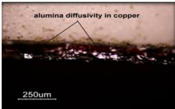
**Fig.(10) Optical microscope image for Copper-alumina in tangential section. (Magnification 100x).**
