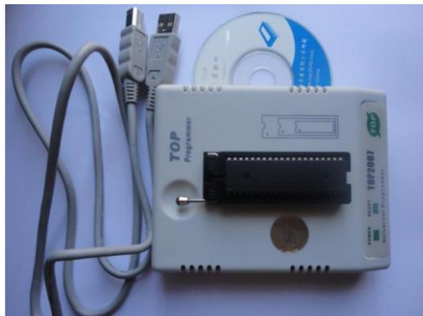
Fig. (2) Top programmer and Topwin<sup>1</sup> program disk.
