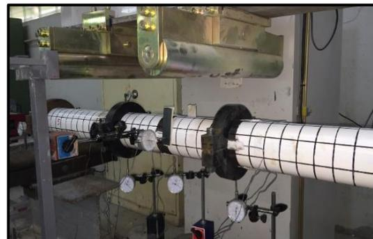
**Figure 3:** Setup of four-point bending test.
