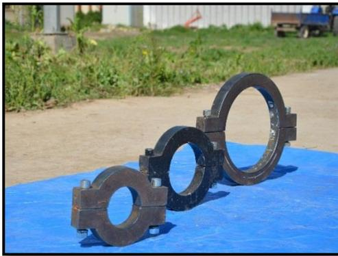
**Figure 1:** Circular collars of the experimental study.
