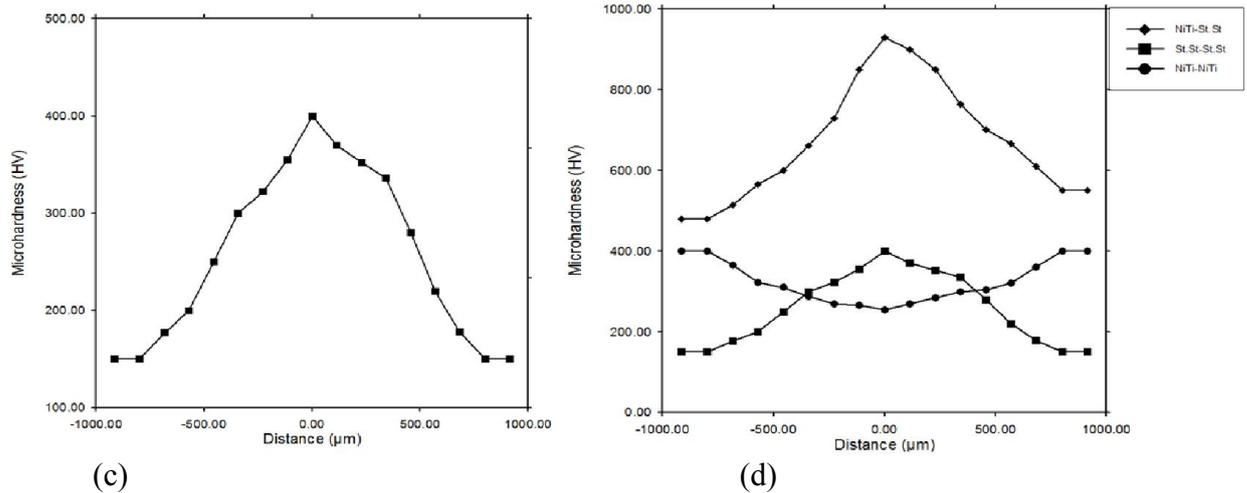
**Fig. (4):** Variation microhardness with distance from weld center (a) NiTi-St.St.(b) NiTi-NiTi (c) St.St.-St.St. (d) NiTi-NiTi, St.St.-St.St. and NiTi-St.St.
