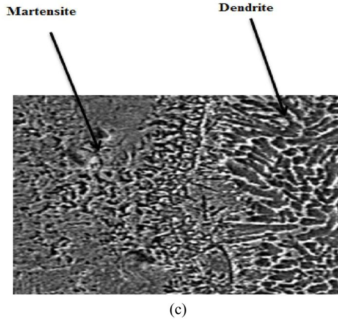
**Fig. (2):**SEM (a) NiTi (BM) (b) NiTi-St.St. (WZ) (c) NiTi-St.St. (Interface)
