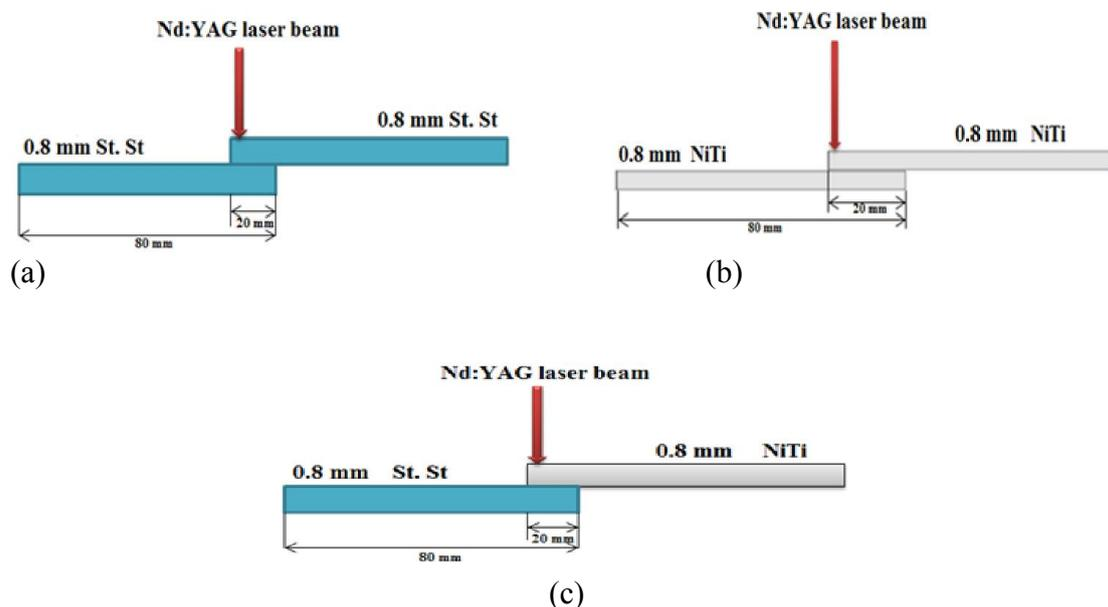
**Fig. (1):** Schematic laser weld (a) St.St.-St.St. (b) NiTi-NiTi (c) St. St.- NiTi
