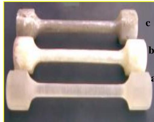
**Fig. (3) A-epoxy , b-epoxy /chopped glass fiber composite c- epoxy /yarn glass fiber composite static torsion specimen.**
