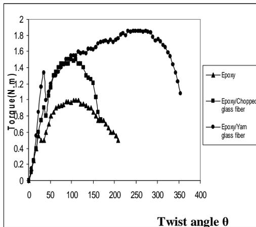
**Fig. (4) Shows the torque- twist angle curves of epoxy and an epoxy chopped , yarn glass fiber rod.**
