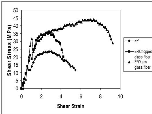
Fig. (5) Shear Stress as a function of Shear strain for epoxy and an epoxy chopped, yarn glass fiber rod.
