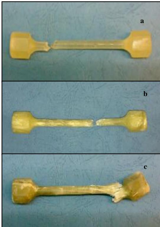
Fig. (6) Failure Modes of (a) epoxy rod (b) Ep/Chopped rod (c) Ep/Yarn rod.
