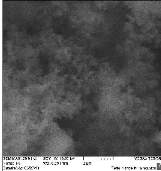
**Figure (2) Scanning Electron Micrograph of Diesel Soot (2  $\mu\text{m}$ ).**
