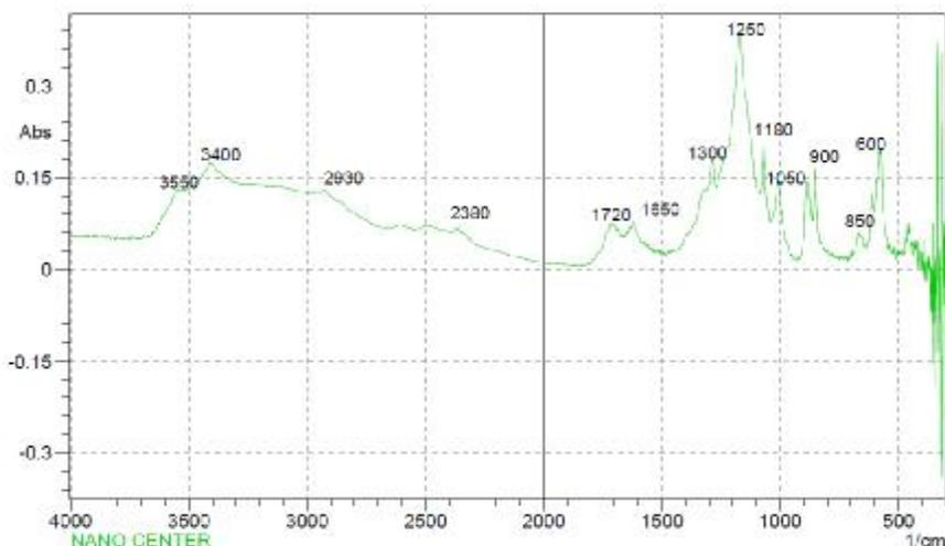
Figure (6) FTIR Spectrum of Soot Obtained.
