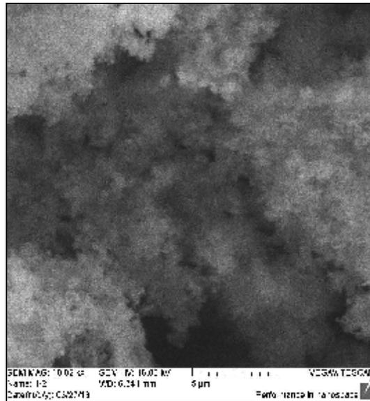
**Figure (3) Scanning Electron Micrograph of Diesel Soot (5  $\mu\text{m}$ ).**
