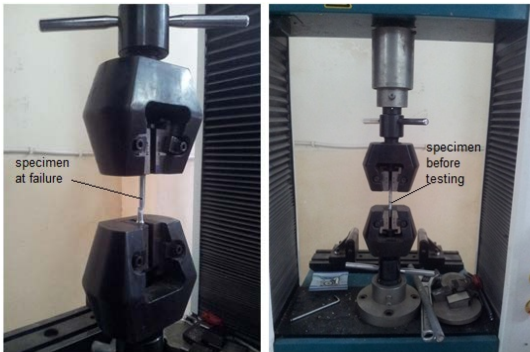
Fig.(1);Tensile test machine in University of Technology with specimen before and after fracture
