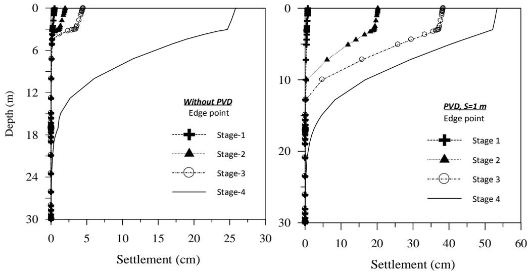
Figure 5: Variation of ground surface settlement under the embankment for treated and untreated soil.
