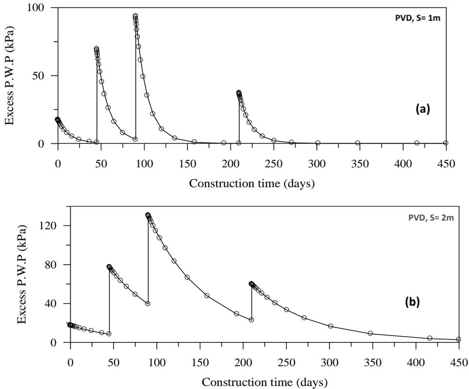
Figure 9: Variation of excess PWP with time under the midpoint of embankment
