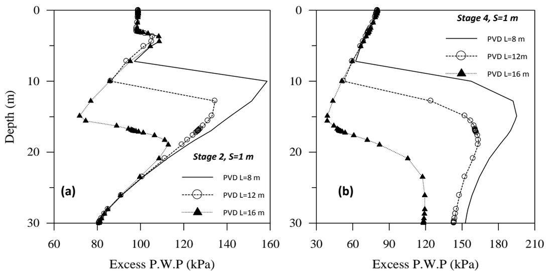
Figure 12: Effect of PVD length on the excess PWP under the midpoint of embankment
