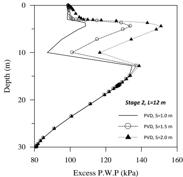
Figure 11: Effect of PVD spacing on the excess PWP under the midpoint of embankment
