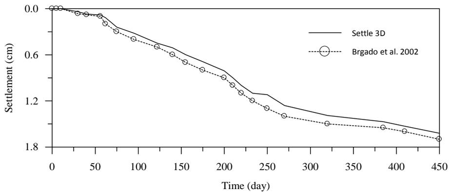
Figure (3) Staged construction of embankment with time
