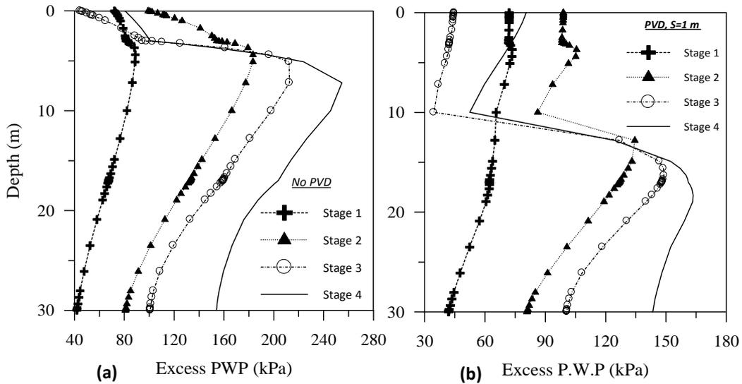
Figure 7: Variation of excess PWP with depth under the midpoint of embankment for treated and untreated soil.
