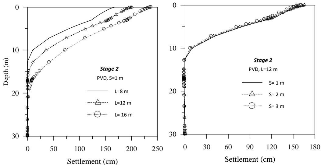
Figure 13: Variation of settlement with depth under different spacing and length of PVD
