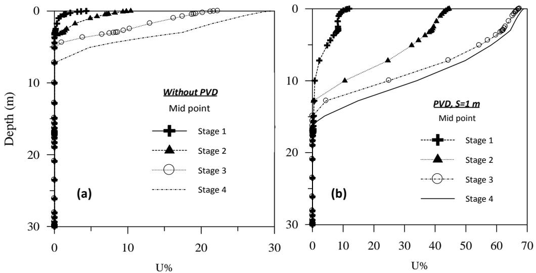
Figure 6: Variation of degree of consolidation with depth under the midpoint of embankment for treated and untreated soil.
