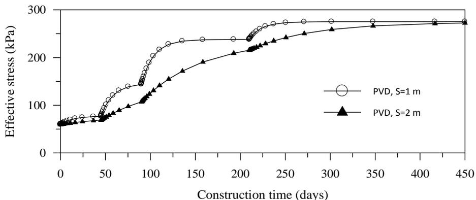
Figure 10: Variation of effective stress with time under the midpoint of embankment.
