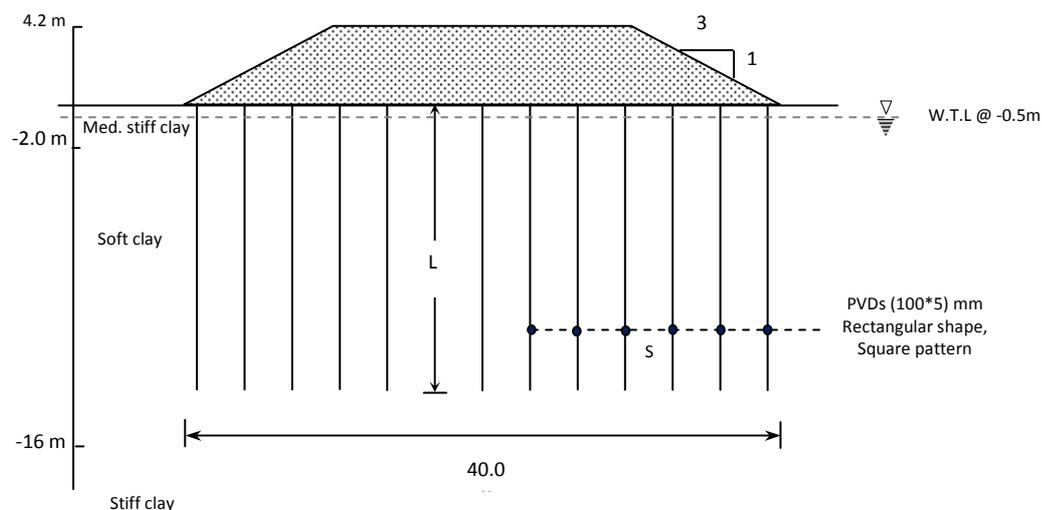
Figure (1) Test embankment on soft clay with PVD and soil profile
