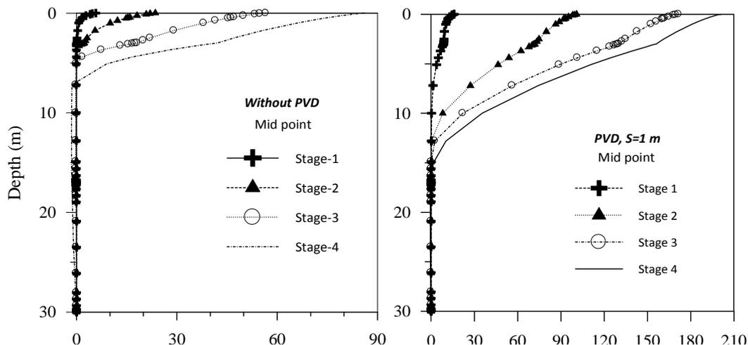
Figure 4: Variation of ground settlement with depth under the midpoint of embankment for treated and untreated soil.
