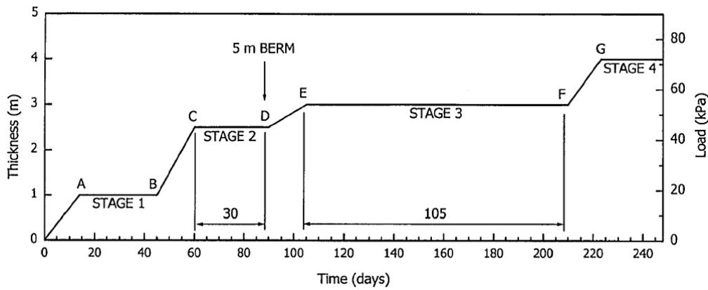
Figure (2) Staged construction of embankment with time
