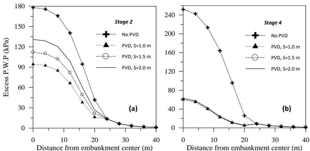
Figure 8: Lateral distribution of excess PWP along ground surface at a depth of 7.0 m under the embankment for treated soil.
