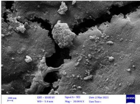
**Figure (5):** The FESEM test Aluminium alloy drilled by pulsed laser and high concentration of silicon carbide nanoparticles (laser energy is 800mJ, frequency is 10Hz, exposure time is 5sec and 90%concentration ratio)
