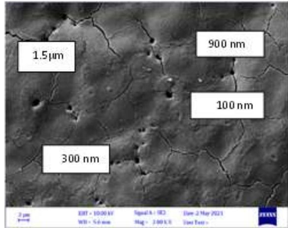
**Figure (9):** The FESEM test of micro holes in aluminium alloy with laser energy of 600mJ, repetition rate is 5Hz, exposure time is 30sec and 50% concentration ratio of nanoparticles
