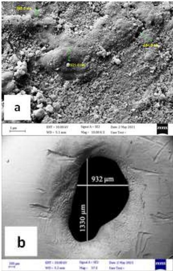
**Figure (8, a-b):** The FESEM test of aggregated nanoparticles and holes in aluminium alloy when the laser energy is 800mJ, repetition rate is 10Hz, exposure is 30sec and 90% concentration ratio of nanoparticles
