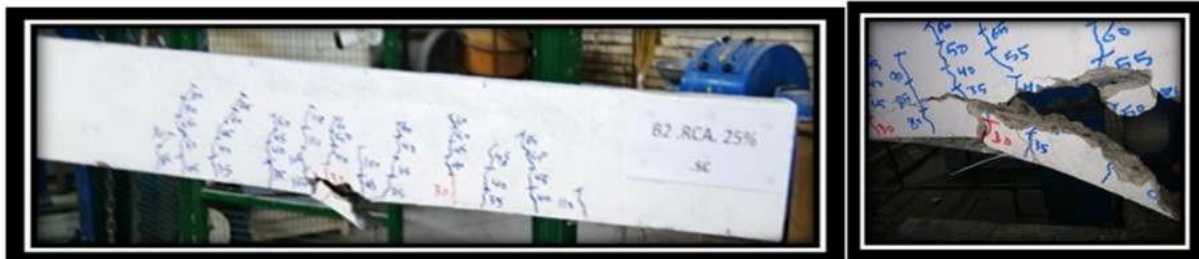
Plate 6. Cracks Pattern of (B2. RCA25%)S.
