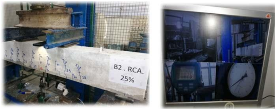
Fig. 3. The Testing of beams specimens.
