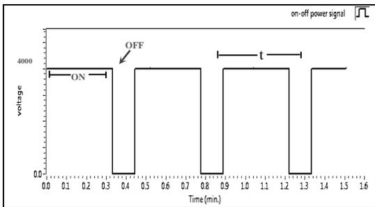
**Fig. 7.** The corresponding ON-OFF time ( $T_1$ ) for defrosting mode, the weight is 100g
