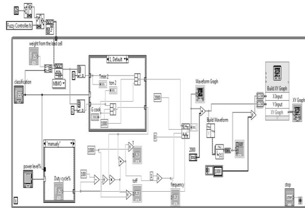
Fig. 3. The block diagram of the designed MWO
