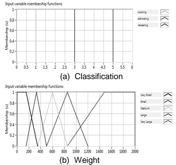
**Fig. 1.** Input variable MFs for the designed FLC
