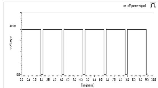
**Fig. 9.** The corresponding ON-OFF time ( $T_1$ ) for reheating mode, the weight is 1000g
