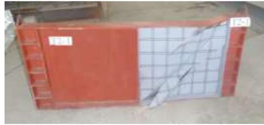
**B) Plate Girder (T2-1) after Testing**
