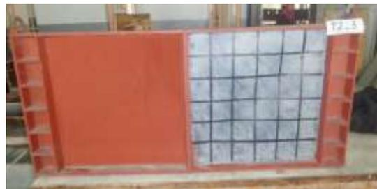
**D) Plate Girder (T2-3) after Testing**
