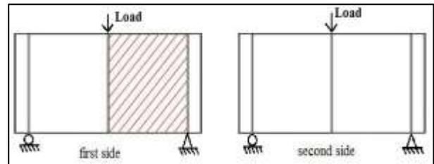
Figure 5: Strengthening technique used for girder (T2-1)
