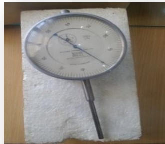
Figure 10: The Dial Gage Used to Monitor Mid Span Deflection
