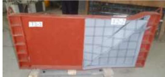
**C) Plate Girder (T2-2) after Testing**
