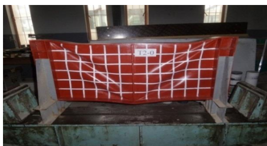
A) Plate Girder (T2-0) after Testing
