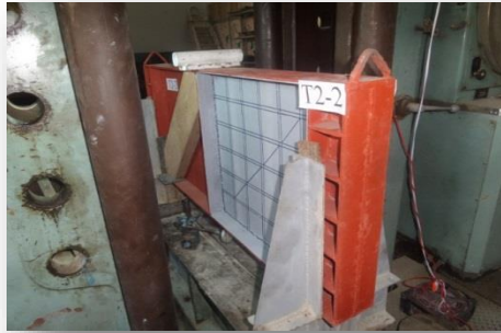
Figure 8: Test Setup of Plate Girder
