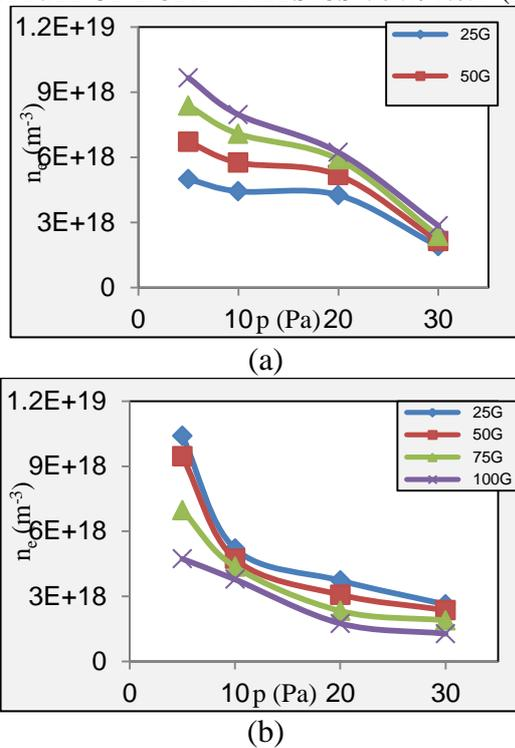
Fig.(6): Electron density variation as function of pressure at different magnetic fields values in presence of (a) longitudinal magnetic field, (b) transverse magnetic field.
