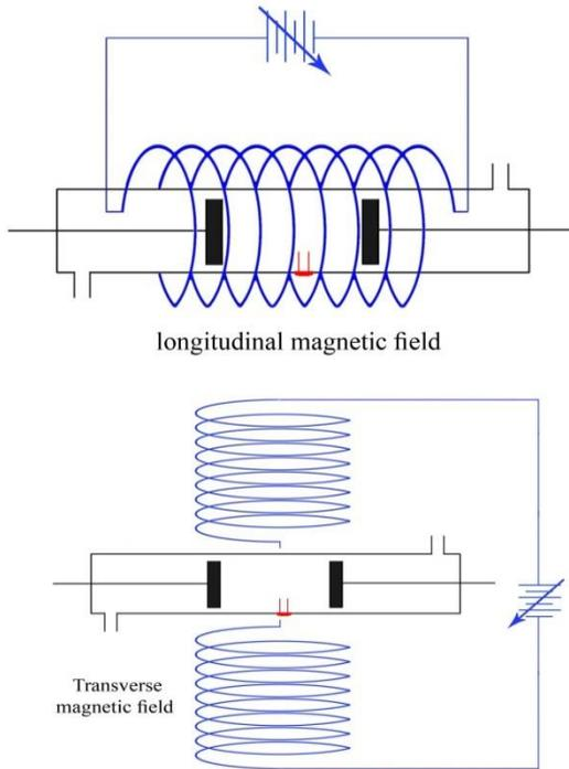
Fig. (2) Discharge tube in longitudinal and transversal magnetic fields.
