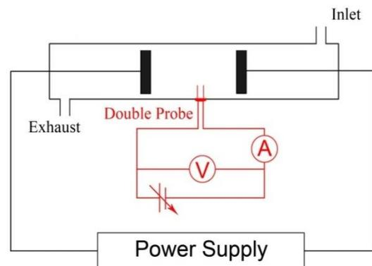
Fig.(1) Shows glow discharge system with probe circuit
