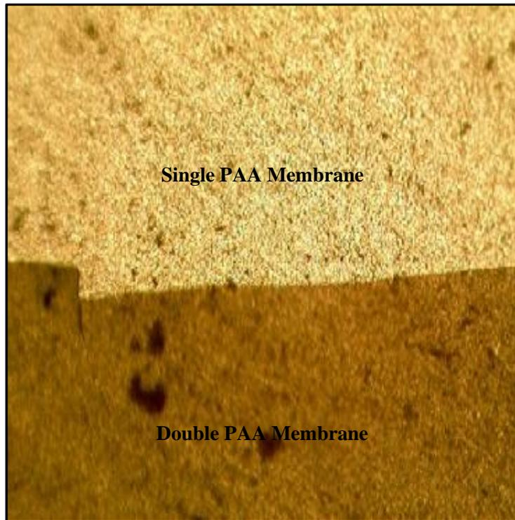
Figure (4) Optical microscopy image of single and Double PAA membrane.
