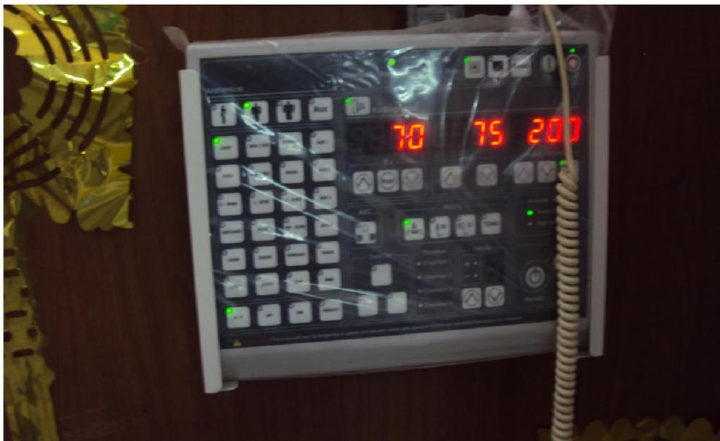
**Fig (1) ;X-ray board control. k.v= 70, time=75, current=200 mA**
