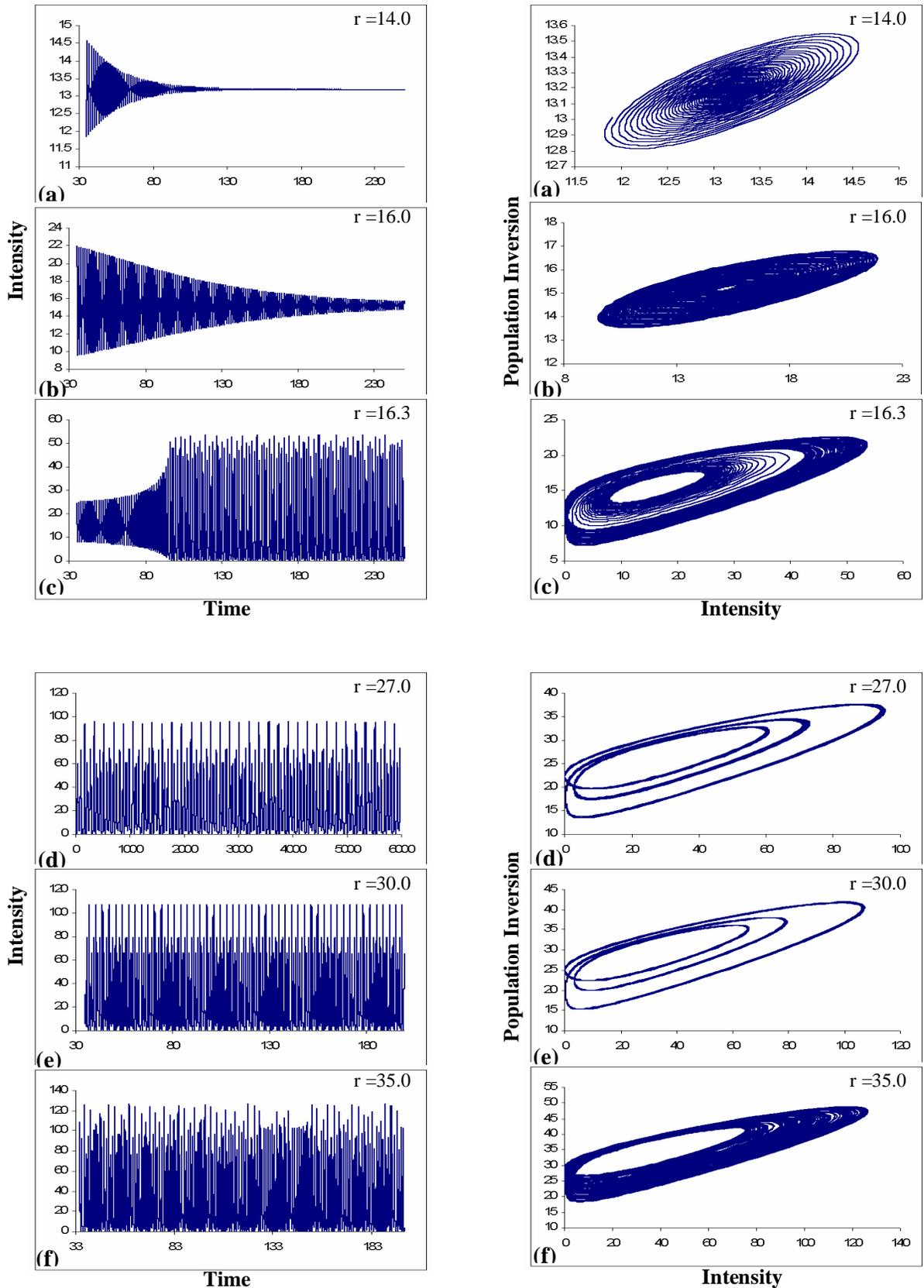
Fig.7. Left side : Intensity time series ( normalized laser field intensity versus normalized time ) at  $\alpha = \theta = 0.5$ ,  $b = 1.0$ , and  $\sigma = 3.0$  for different values of  $r$ . Right side : The corresponding phase – space portraits ( laser field intensity against population inversion ).
