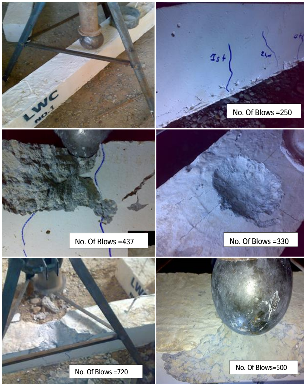
Figure (12) Number of blows from first crack up to failure for lightweight Concrete beam
