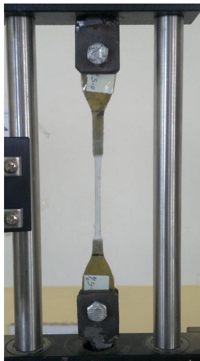
Fig. 5. Ductility of PP
