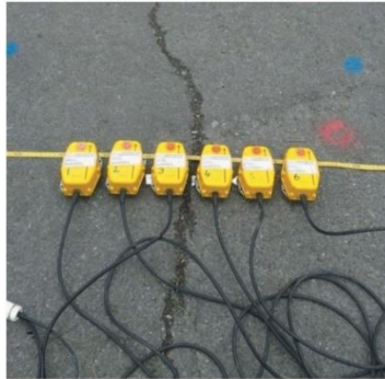
Fig. 8. Use of Raleigh Wave method for detecting crack propagation. Taken from. (Iodice et al., 2020).
