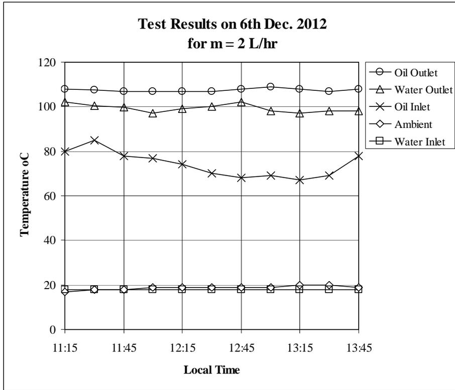
Fig .(6) Variation of oil an water temperatures for a mass flow rate of 2 L/hr.
