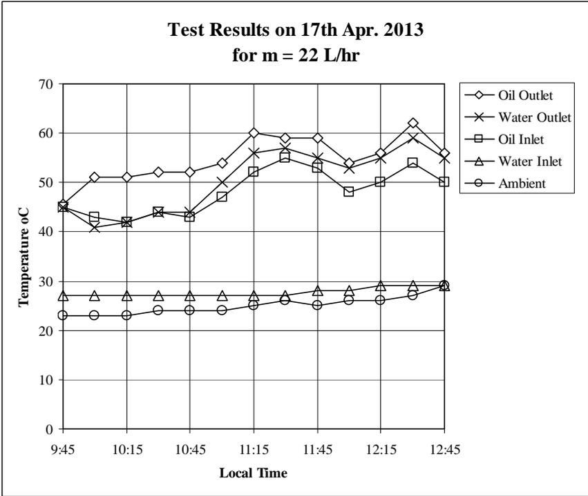
Fig .(9) Variation of oil an water temperatures for a mass flow rate of 22 L/hr.
