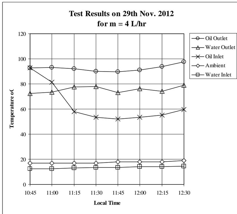
**Fig .(5) Variation of oil an water temperatures for a mass flow rate of 4 L/hr.**
