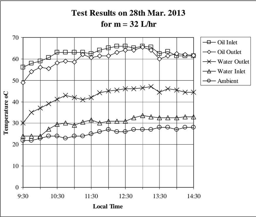
Fig .(8) Variation of oil an water temperatures for a mass flow rate of 32 L/hr.
