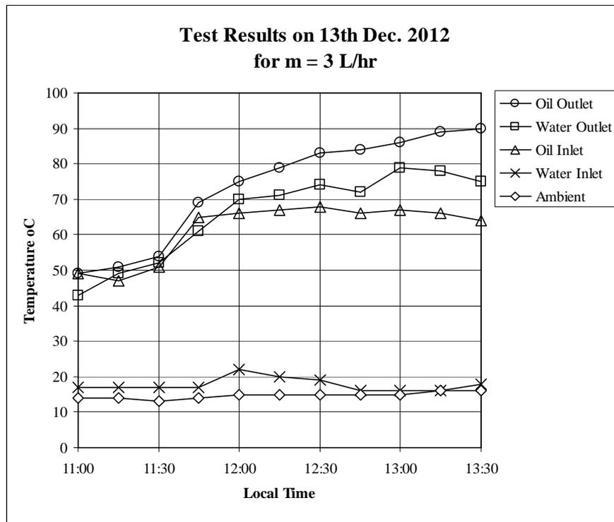
Fig .(7) Variation of oil an water temperatures for a mass flow rate of 3 L/hr.
