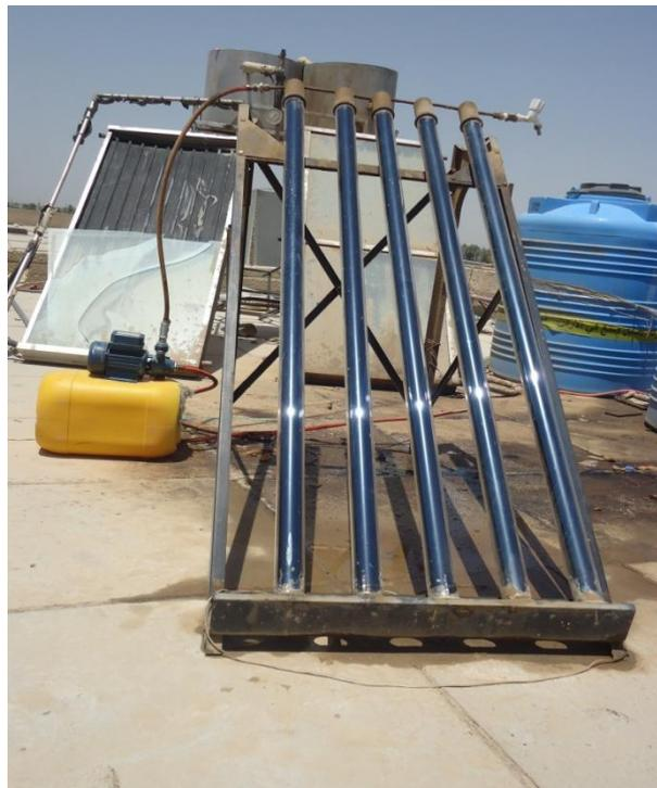
**Fig .(2) The evacuated-tube solar collector under study.**
