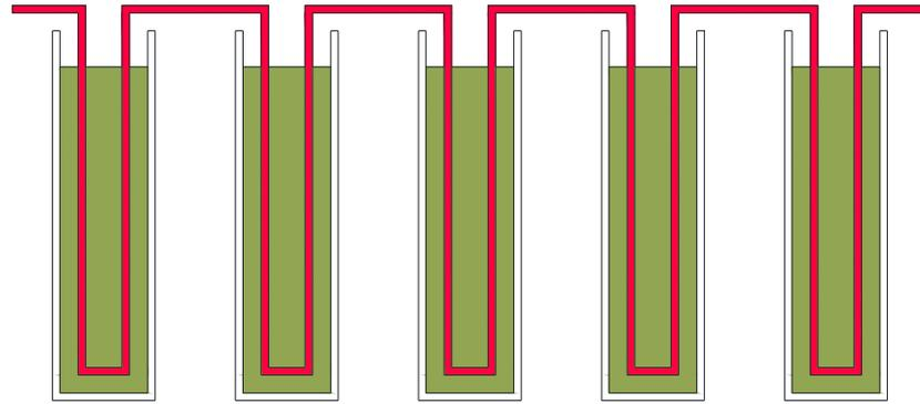
**Fig .(3) Schematic view illustrating the steel pipe (red) immersed in the oil (green).**
